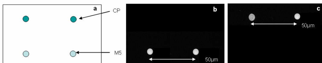
Figure 3.29: (a) Schematic of a fabricated polypyrrole-ODN matrix composed of one row of CP and one row of M5 ODN. (b) Fluorescence picture after hybridization with M5 complementary strand at 0.1 \mu\text{M} . (c) Fluorescence picture after hybridization with CP complementary strand at 0.1 \mu\text{M} .
