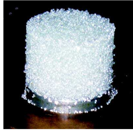
Fig. 11. Sample composed of glass beads prepared for axial-compression test.
