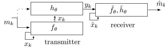
FIG. 2.7 – Message-embedding.  $m_k$  is embedded into  $f_\theta$  and  $h_\theta$  if the inherent delay is 0 or  $m_k$  is only embedded into  $f_\theta$  if the inherent delay is strictly greater than 0
