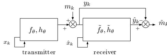
FIG. 2.3 – Additive masking
