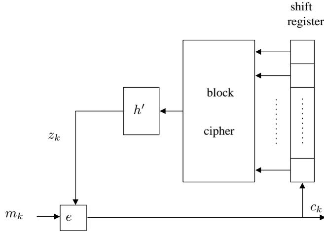
FIG. 4.2 – Block cipher in CFB mode
