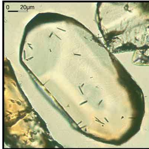
Fig. 3.2. Spontaneous fission track in apatite crystal. Magnification 1250X.
