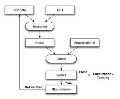
Figure 2.1 – Software Testing Process
