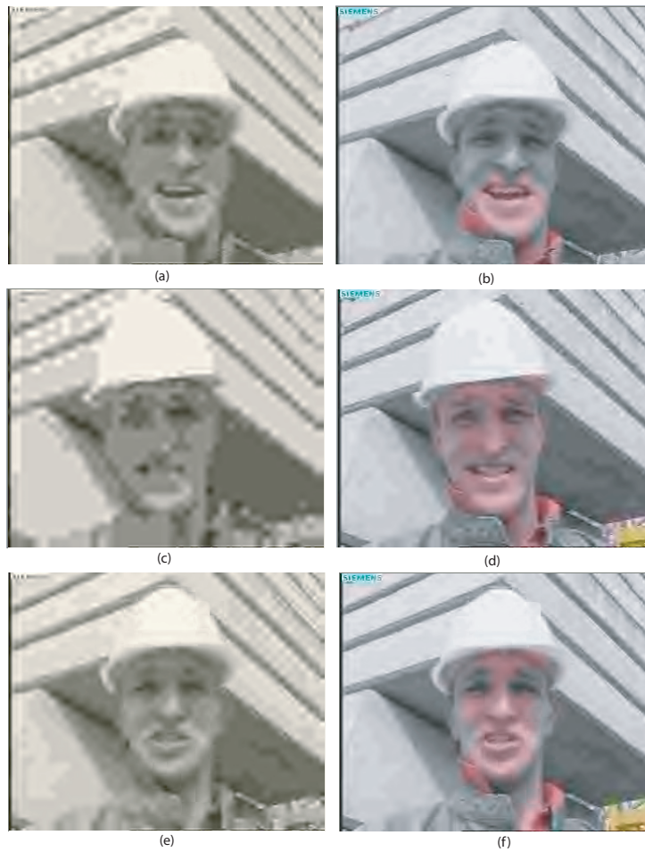
Figure 3.17: Decoded FOREMAN at 200 Kbps ; images 20, 45 and 54; (a), (c), (e): half-pixel accuracy with vectors coded losslessly ( R_v = 143.4 Kbps) ; (b), (d), (f): half-pixel accuracy with the bit allocation approach and motion vectors quantized at R_v^* = 48.5 Kbps.
