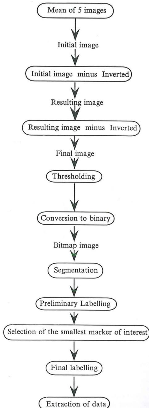
FIG. 2. Image processing algorithm.
