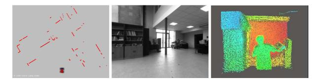
Figure 1.3: Perception of the same environment with a laser-range scanner (left) and a camera (centre). Right: depth image acquired with a Swissranger sensor.
