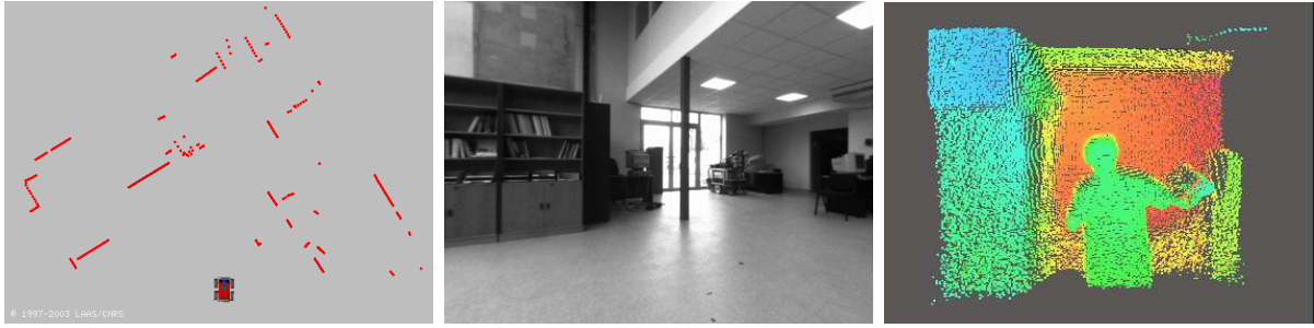
Figure 1.3: Perception of the same environment with a laser-range scanner (left) and a camera (centre). Right: depth image acquired with a Swissranger sensor.
