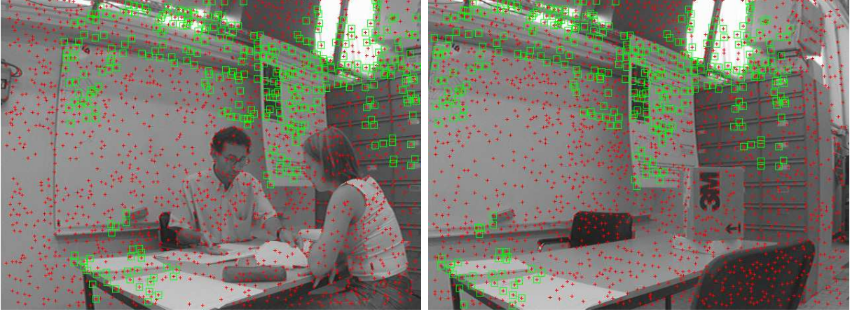
Figure 3.2: Results of the matching algorithm. The red crosses shows the interest points, the green squares indicate successful matches. There was 194 matches for a total computational time of 201ms (including 116ms for the Harris points detection and 85ms for the matching) from [LBJL06].
