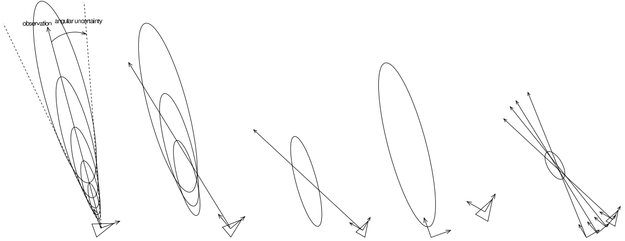
Figure 2.3: From an observed feature to a landmark in the map. From left to right: the sum of Gaussians is initialised in the robot frame; some Gaussians are pruned based on their likelihood after additional observations of the feature; when a single hypothesis remains, the feature is declared as a landmark and it is projected into the map frame; and finally past observations are used to update the landmark estimate.
