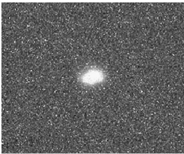
Fig. 6. Radioluminescence emission of A-sub sample during 6 MeV photon beam irradiation.
