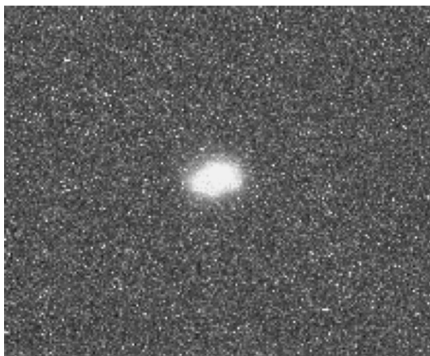
Fig. 1. Photograph of a Si-doped GaN sample under 6 MV photon beam radiation with integration time of 10 s.
