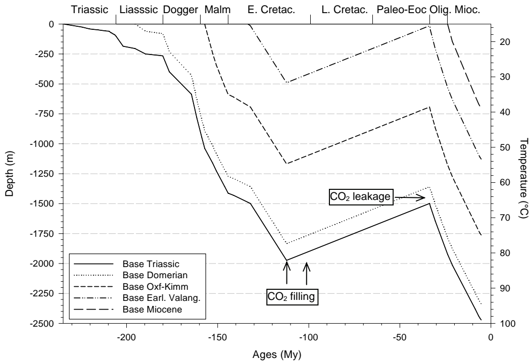
Figure 60 - Burial curves of sedimentary formations of Valence Basin and the filling phase of Montmiral sedimentary CO 2 reservoir CO 2 leakage corresponds to carbonic inclusions observed in Hettangian formation (Shepherd, 2003).
