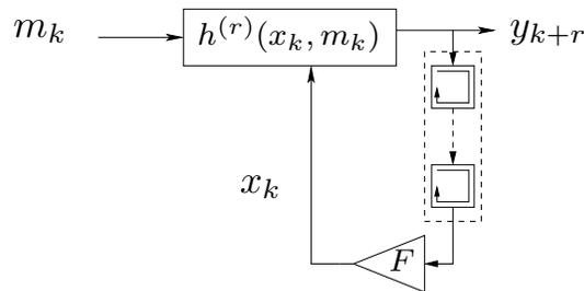
FIGURE 4.1 – Self-synchronizing Message Embedded Stream Cipher
