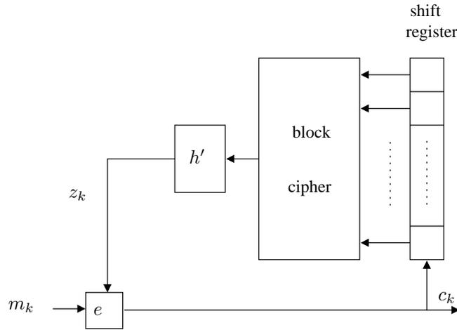
FIGURE 4.2 – Block cipher in CFB mode
