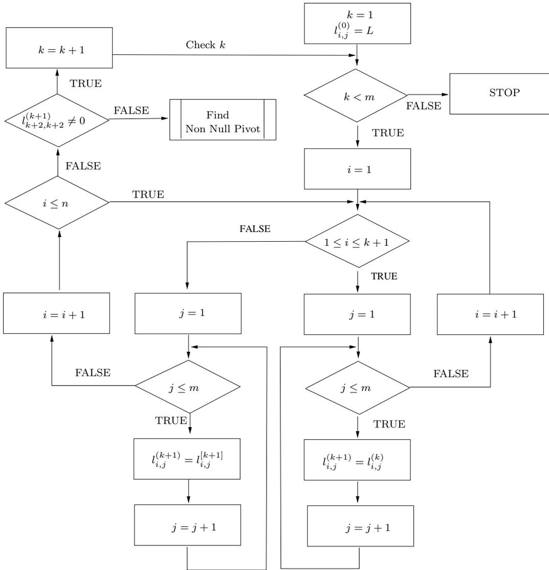
FIGURE C.1 – Diagram detailing the Gaussian-Bareiss elimination method
