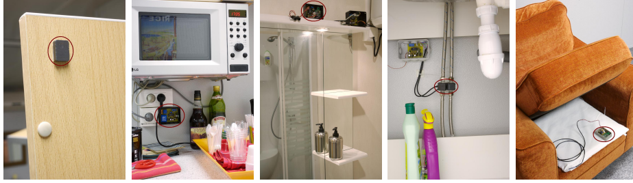
Figure 6.6: Views of some environmental sensors installed in the Gerhome laboratory. Sensors are circled. (a) Contact sensor on cupboard door in the kitchen; (b) Electrical sensor on electrical outlet in the kitchen; (c) Presence sensor in front of the washbowl in the bathroom; (d) Water sensor on water pipe in the kitchen; (e) Pressure sensor under the armchair in the livingroom.
