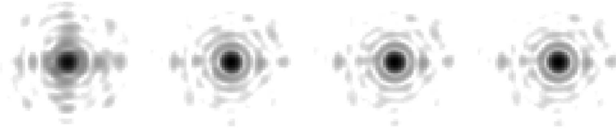
Fig. 9. Focused images obtained on the ONERAAO bench (logarithmic scale) corresponding to the first four points of Fig. 8. The image on the left is the image obtained without any precompensation. The SR of the last image is 93.8%. Conditions are the same as in Fig. 6.
