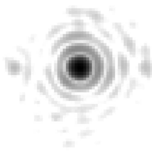
Fig. 12. PSF obtained after three iterations of NCPA precompensation. 42 modes are compensated (from Z_4 to Z_{45} ), and the exact value of a_4 has been optimized. SR is 98.7%, \lambda=632.8 nm.
