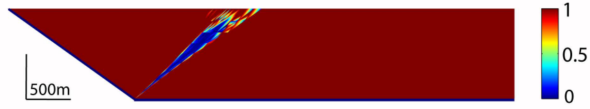
FIG. 2.16: The failure mode in the fault-bend fold without relief build up with a ramp dipping at \gamma = 35^\circ , \phi_R = 15^\circ , defined by the scaled distance to the criterion. The blue line marks the activation of the ramp and the décollement. Note the absence of any failure other than the back thrust in the bulk.
