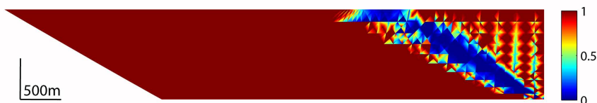
FIG. 2.15: The pre-defined ramp is not used for the fault-bend fold without relief build up for \phi_R = 15^\circ , as revealed by the scaled distance to the Coulomb's criterion ( \phi_D = 10^\circ, \gamma = 30^\circ ).
