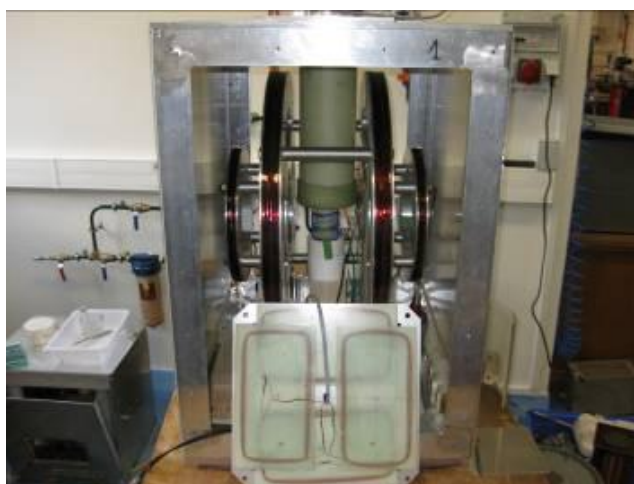
Figure 46: Picture of the MRI experimental setup built in our laboratory. The static field is generated by the largest copper coils. Smaller coils are the shimming coils. Gradients coils can be seen in front of the picture. A 5 \times 5 \times 5 \text{ cm}^3 volume can be scanned in this setup.
