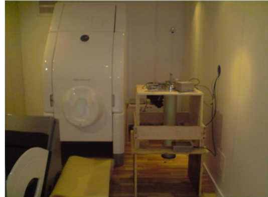
Figure 23 : Left: Schematic of the MCG experiment. Right: Picture of the experimental setup (fiberglass dewar and low-noise amplifier) on the right in Neurospin MSR. The commercial MEG system is visible on the left of the picture.
