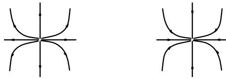
FIG. 7.36: Noeud impropre instable et Noeud impropre stable
