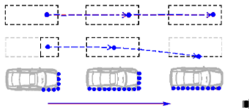
(b) when moving, vehicle comes in different size (visible parts) which degrades the tracking result
