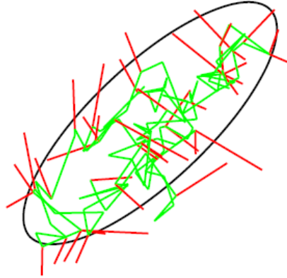
Figure 4.8: A simple illustration of Metropolis algorithm to sample from a Gaussian distribution whose one standard-deviation contour is shown by the ellipse. Steps that are accepted are shown in green and rejected steps are shown in red.
