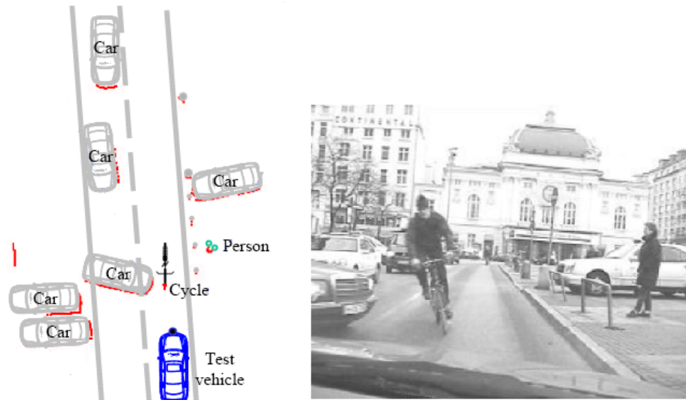
Figure 1.2: The ultimate goal of vehicle perception including fundamental tasks: Localization, mapping with detection, classification and tracking moving objects.
