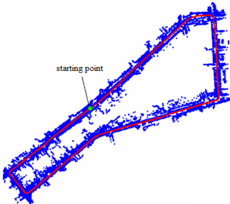
Figure 3.13: The result of localization compared with the ground-truth map.
