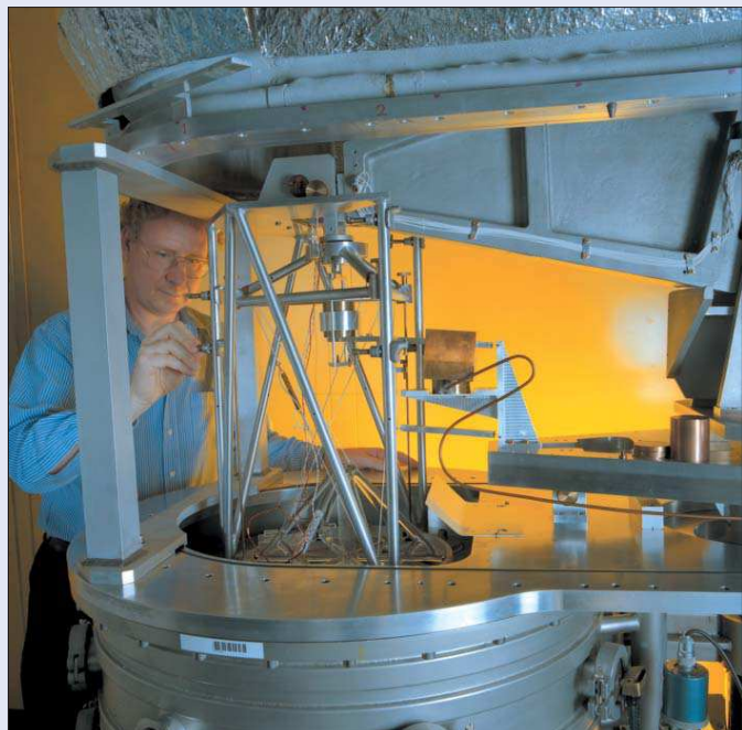
Well balanced Using a watt balance, like this one at the National Physical Laboratory in the UK, requires a precise knowledge of the local acceleration due to gravity.
