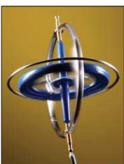
In a spin Conventional mechanical gyroscopes use the forces on a spinning flywheel to measure rotations.
