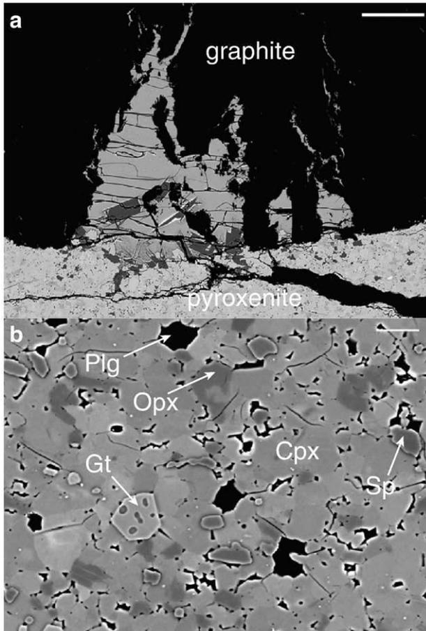
**Fig. 2.** Backscattered electron micrographs illustrating the melt extraction technique. (a) An overall view of the lower part of sample 40-F2, showing the graphite container (black), the partially molten pyroxenite (grey), and a basaltic microdike showing a large pool of glass. (b) Close-up view of the partially molten pyroxenite showing a small fraction of interstitial melt (3.4 wt.%) in equilibrium with Cpx, Opx, Plg, Sp and Gt. Scales: 100  $\mu\text{m}$  in (a); 10  $\mu\text{m}$  in (b).
