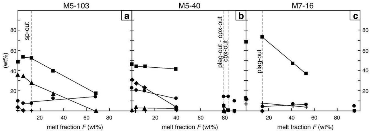
**Fig. 4.** Fractions (wt%) of solid phases vs. melt fraction  $F$  for pyroxenites (a) M5-103, (b) M5-40, and (c) M7-16 at 1 GPa. The straight lines are the best fit lines used to compute the coefficients of the melting reactions. Symbols are as follows: squares for Cpx, triangles for Opx, circles for Ol, diamonds for Plg and crosses for Sp. The uncertainties on phase percentages are given in Table 2.
