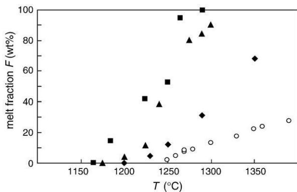
**Fig. 3.** Temperature–melt fraction curves for pyroxenites M5–103 (diamonds), M5–40 (triangles) and M7–16 (squares) at 1 GPa; the data for fertile lherzolite MM3 (circles; Baker and Stolper, 1994; Baker et al., 1995) are shown for comparison. The uncertainties on melt percentages ( $1\sigma$ ) are smaller than symbols.
