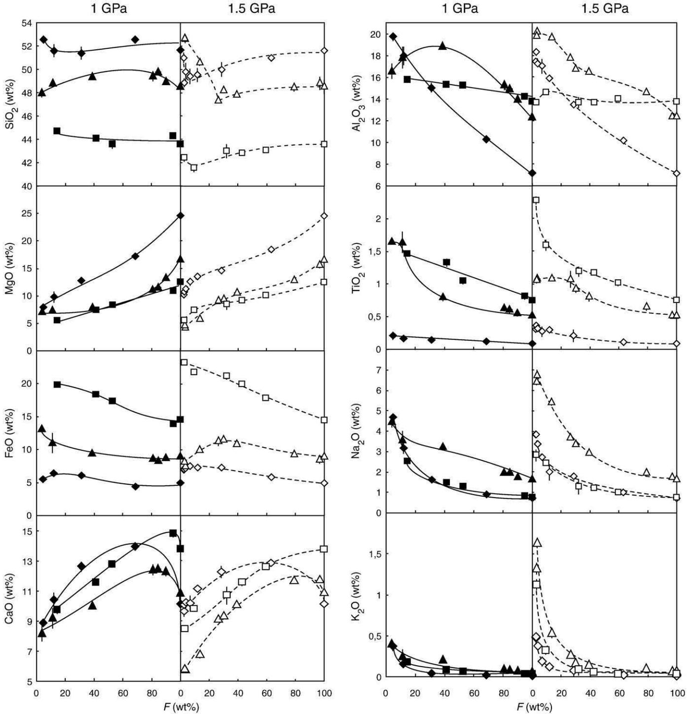
**Fig. 5.** Oxide concentrations in melts plotted as a function of melt fractions  $F$ . Symbols are as follows: diamonds for pyroxenite M5–103, triangles for M5–40, and squares for M7–16; the closed symbols are for the experiments at 1 GPa, the open symbols for the ones at 1.5 GPa. The data plotted at  $F=100\%$  correspond to the bulk-rock composition. When not visible, the error bar ( $1\sigma$ ) is smaller than the symbol.
