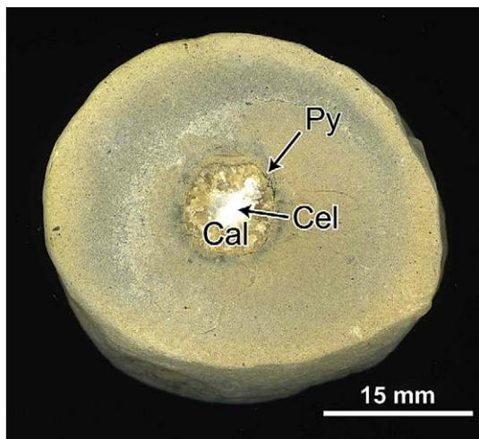
**Fig. 8.** Section of a small tubular concretion found near Pr15. The central conduit is probably an initially empty *Paratiosa contorta* bioturbation (Gaillard, 1972). The conduit partly bounded by pyrite (Py) is then filled by dogtooth brown calcite (Cal) and by subhedral pure celestite (Cel). Small fractures filled with brown calcite can be seen around the central conduit. Colour variations of the concretion, due to weathering, are also easily observable.
