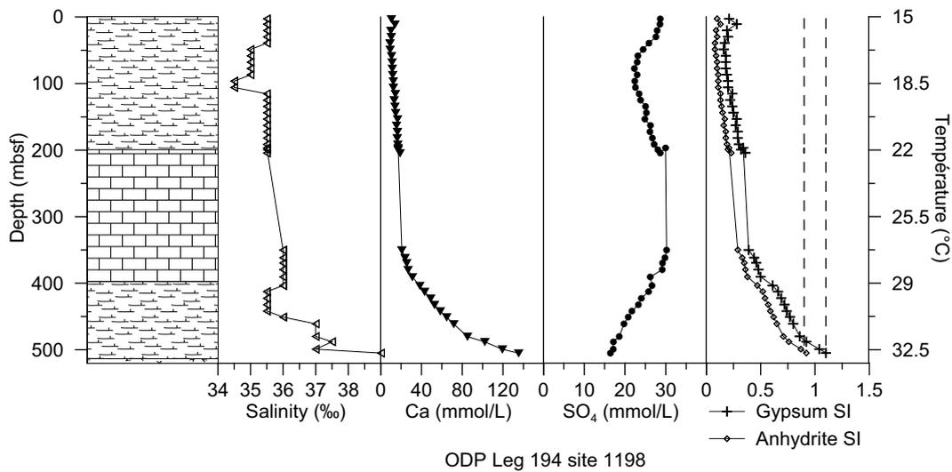
**Figure 5.6.** The simplified lithology (left column), variation of porewater salinity, Ca and SO<sub>4</sub> concentrations, and the gypsum and anhydrite saturation indices versus depth for ODP Leg 194 site 1198.
