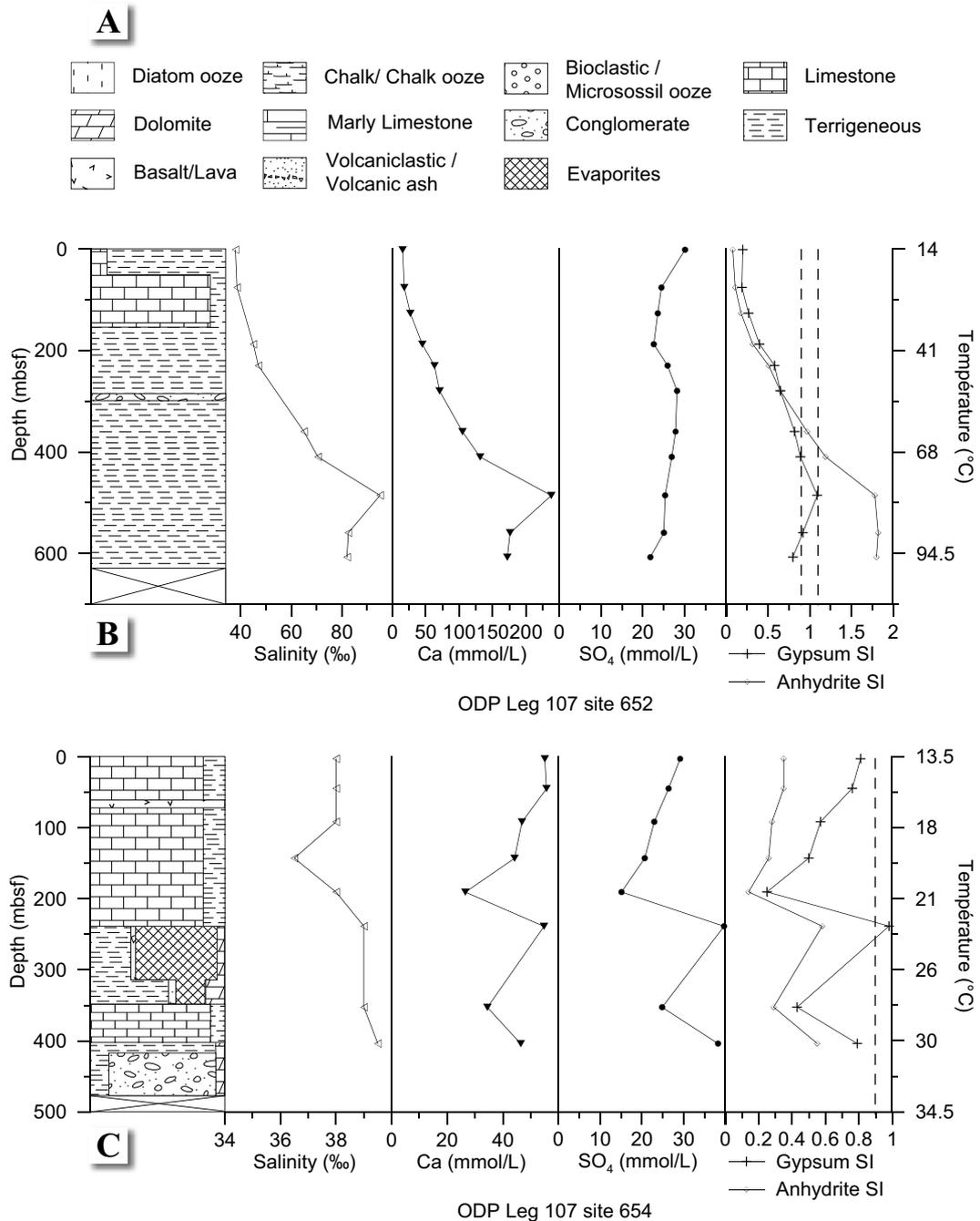
**Figure 5.2.** (A) Graphic symbols used for the lithological description of sites (all figures); (B), (C). The simplified lithology (left column), variation of porewater salinity, Ca and SO<sub>4</sub> concentrations, and the gypsum and anhydrite saturation indices versus depth for ODP Leg 107 sites 652 (B) and 654 (C). Equilibrium is reached between the dashed lines (saturation index values between 0.9 and 1.1).
