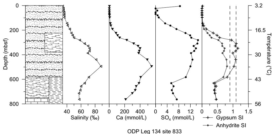
**Figure 5.5.** The simplified lithology (left column), variation of porewater salinity, Ca and  $\text{SO}_4$  concentrations, and the gypsum and anhydrite saturation indices versus depth for ODP Leg 134 site 833.
