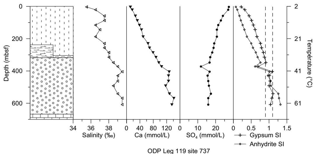
**Figure 5.9.** The simplified lithology (left column), variation of porewater salinity, Ca and  $\text{SO}_4$  concentrations, and the gypsum and anhydrite saturation indices versus depth for ODP Leg 119 site 737.
