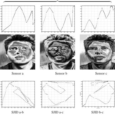
Figure 1.4: Synthetic sensors and the support of the joint intensity distribution (SJID) of their outputs. The second and third rows represent the response and output of three synthetic sensors.
