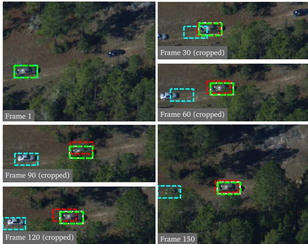
Figure 9.2 – Tracking on sequence “Car” (frame indices are relative to the reference frame). Green • kNN-KL-G (proposed method), Cyan • kNN-KL, Magenta • Pz-KL-G, Red • Mean-Shift, Black • SAD (white on the frames and black in the diagram). There are several frame drops at frame 38 (vertical dashed line in the diagram) and the tracked car is partially occluded by trees from frame 42 to frame 122 (gray area in the diagram). \Omega : 95 \times 47 -rectangle – Figure continued in Fig. 9.3.
