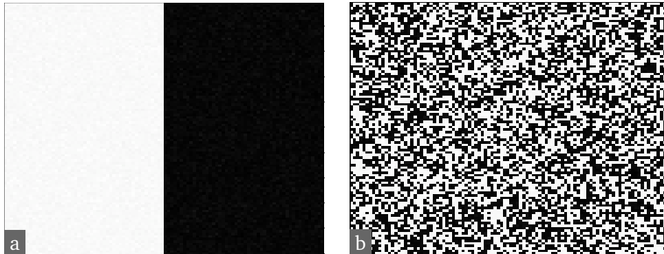
Figure 2.6 – Two images with equal entropy ([b] was obtained by scrambling the pixels of [a]). As is clear from these images, piecewise constant and minimal (pixel-level) entropy are not synonymous.
