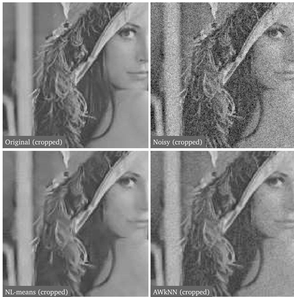
Figure 8.6 – Denoising of the image “Lena”. The homogeneous areas are well recovered by NL-means whereas AWkNN better preserves the textures.
