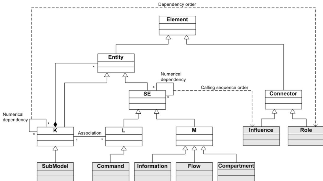
**Fig. 1.** Class diagram of SIMILE language designed using the UML convention. Classes are represented by rectangles. Classes in grey correspond to those being instantiated by the user. The diagram was inferred from the description of functionalities by [5].
