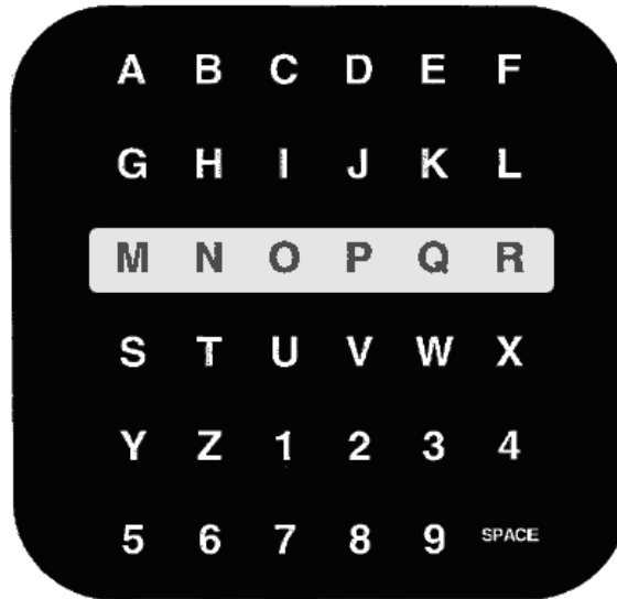
Figure 2.3: In the P300 speller by Farwell and Donchin [32], items are presented on a 6 by 6 matrix. Rows and columns are flashed in a random sequence, eliciting a P300 signal 300 ms after the key the user wants to select has been flashed.
