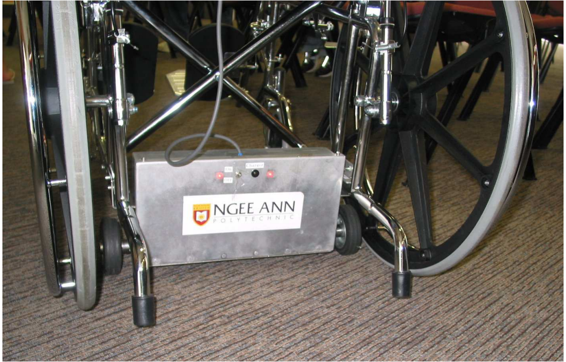
Figure 8.3: A wheelchair powering module by Ngee Ann Polytechnic, Singapore.
