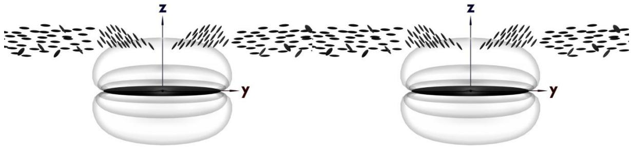
**Figure 7.7-** Pictographic representation showing the whole scenario found in the sample.  $\{111\}$  particular arrangements of  $H$ -platelets are created above the  $He$ -plates, and  $(001)$   $H$ -platelets are formed in the zones far from  $He$ -plates. The distance between each arranged nano-domain exceeds its average diameter.
