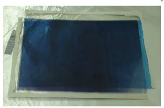
Figure IV.7: Application (manual lamination) of coloured PEDOT on the electrolyte/Prussian Blue stacks.
