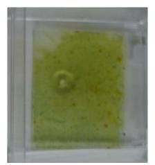
Figure E.2: Example of deposition using spin coating, 1000 pm, 30s.
