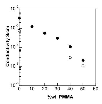
Figure II.42: Conductivity at 293 K of PMMA membranes plasticized by (1-x)(BMITFSI), xLiTFSI ionic liquids containing LiTFSI mole fractions x = 0.03 (filled circle) and 0.23 (open circle).
