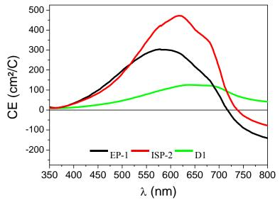
Figure III.16: Colouration efficiency of PEDOT films on FTO/glass
