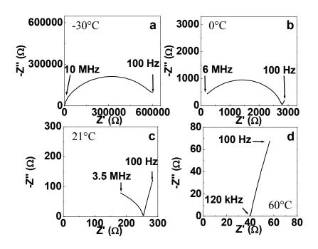
Figure II.13: EIS spectra of a cell containing the gel electrolyte BMITFSI /  $x_{\rm LiTFSI}$  = 0.03 / PMMA =40 wt% in between two stainless-steel electrodes for different temperatures : (a) - 30 °C, (b) 0 °C, (c) 21 °C, (d) 60 °C
