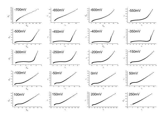
Figure F.2 : EIS spectra of a Prussian Blue film at 3 mC/cm<sup>2</sup> on a FTO/glass electrode. The potential increases from – 700mV to + 250 mV.
