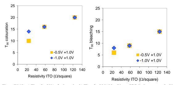
Figure IV.19 : a) Time for 90% of colouration b) Time for 90 % bleaching, of EC devices prepared with conducting substrate of sheet resistance 24, 58 and 124  $\Omega/\Box$  : colouration at -0.5V and at -1V.0 for 30 s. followed by bleaching at 1.0V the next 30 s.
