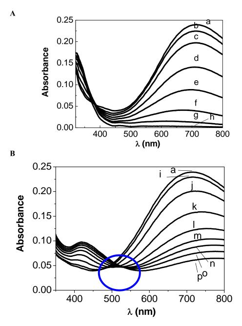
Figure III.26: Absorbance of a Prussian Blue film at 3 mC/cm² on FTO/glass for different applied potential, ref Ag/AgCl, CE=Pt wire. A: Reduction of Prussian Blue: a)0.5V, b) 0.3V, c)0.2V, d) 0.1V, e) 0V, f) -0.1V, g) -0.2V, h) -1 V; B: Oxidation of Prussian Blue: a) 0.5V, i) 0.6V, j) 0.7V, k) 0.8V, l) 0.9V, m) 1V, n) 1.1V, o) 1.2V, p) 1.3V.
