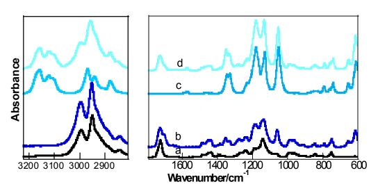
Figure II.28: ATR-IR spectra at room temperature of PMMA: (a), of a LiTFSI/PMMA blend with MMA/Li = 9.5: (b), of the 0.77(BMITFSI),0.23 LiTFSI ionic liquid: (c) and of PMMA (40 wt%) plasticized by 0.77(BMITFSI),0.23 LiTFSI: (d). The intensities between 3200 and 2800 cm<sup>-1</sup> have been amplified by a factor of about 20.
