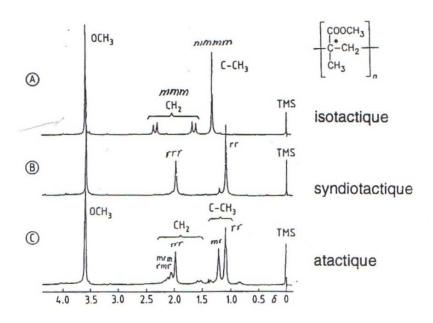
Figure D.5: 1H RMN spectra at 220MHz. Solution of poly(methyl methacrylate) in odichlorobenzene at 100°C.
