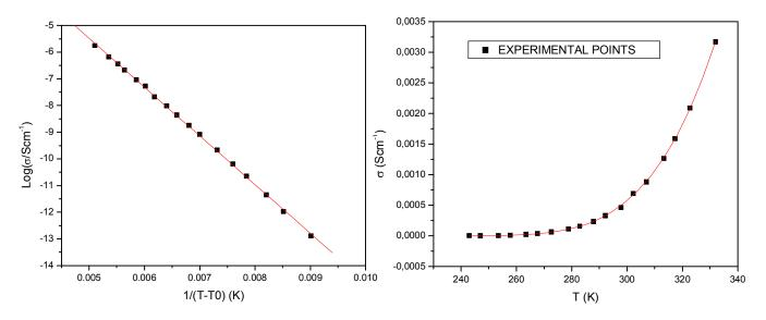
Figure II.15: Temperature dependence simulation of the conductivity  $\sigma$  in the range -30°C - +60°C for a BMITFSI solution with LiTFSI molar fraction of 0.36. a)  $Log(\sigma T) = f(1/(T-T_0), b) \sigma = f(T)$ ; the red line is the VTF fit.
