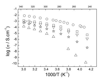
Figure II.23: Temperature dependence of the ionic conductivity  $\sigma$  for BMITFSI electrolytes with LiTFSI molar ratio of x = 0.03 and PMMA wt%:  $\bigcirc 0\%$ ;  $\square 20\%$ ;  $\nabla 30\%$ ;  $\stackrel{\checkmark}{\triangleright} 40\%$ ,  $\triangle 50\%$
