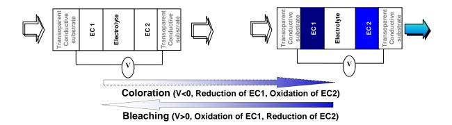
Figure I.6: Working-principle of an ECD (electrochromic device).
