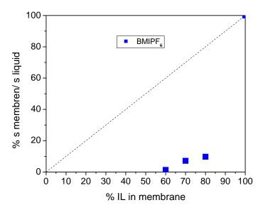
Figure C.5: Evolution of  $\sigma_{membrane}/\sigma_{liquid}$  as compared to the wt% of liquid in the membrane
