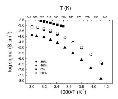
Figure C.4 : Temperature dependence of the conductivity  $\sigma$  for pure BMIPF<sub>6</sub> electrolytes with PMMA wt%:  $\blacksquare$  0%; o: 20%,  $\bullet$  30%;  $\blacktriangle$  40%.
