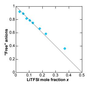
Figure II.33: Population of 'free" TFSI anions in (1-x)(BMI-TFSI),xLiTFSI ionic liquids evaluated from the fraction of intensity contained in the 742 cm<sup>-1</sup> component of Figure II.32. A theoretical line of slope -2 is drawn for comparison.
