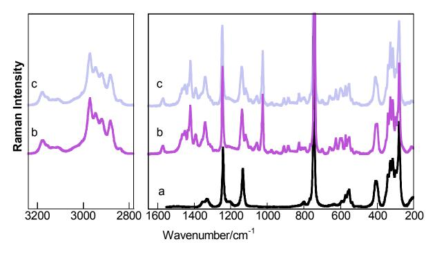
Figure II.30: Raman spectra at 298 K of an aqueous solution of LiTFSI (a), of the ionic liquid BMITFSI (b), and 0.77(BMITFSI),0.23LiTFSI (c).
