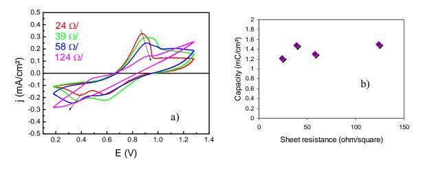
Figure III.23: Electrodeposition of InHCF on ITO substrates on glass with different sheet resistances (24 to  $124\Omega/\Box$ ). a) Last electrodeposition voltammetric cycle (50<sup>th</sup>); b) capacities measured from the area of the cyclic voltammogram on the last deposition cycle.
