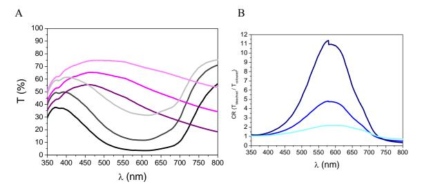
Figure III.9 : A) Transmittance spectra recorded for electropolymerised PEDOT films EP1 (light), EP2 (medium) and EP3 (dark). The pink lines correspond to the bleached state (once oxidised at 1.0  $V_{Ag/AgCl}$ ) and the grey lines to the coloured states (once reduced at -1.0  $V_{Ag/AgCl}$ ) in 0.03LiTFSI/0.97 BMITFSI (molar ratio) electrolyte. B) Contrast ratio for these films EP1 (light), EP2 (medium) and EP3 (dark)
