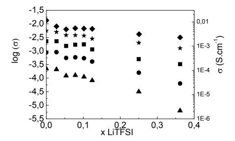
Figure II.16: Variation of the conductivity  $\sigma$  (S.cm<sup>-1</sup>) of the electrolyte with the LiTFSI in BMITFSI molar fraction (x=0 to x=0.36) for temperatures:  $\blacktriangle$  -20°C;  $\blacksquare$  20°C;  $\bigstar$  40°C;  $\spadesuit$  60°C
