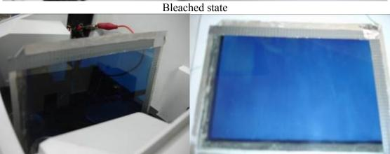
Figure IV.21 : Bleached and coloured state of the complete device, on the left view of the spectrophotometer installation for transmission measurements.
