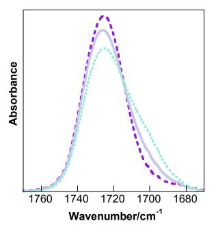
Figure II.43: Infrared spectra in the C=O stretching vibration of PMMA (40 wt%) plasticized by (1-x)(BMI-TFSI), LiTFSI ionic liquids containing LiTFSI mole fractions of x = 0.028, 0.23 and 0.37, by order of decreasing intensity at 1729 cm<sup>-1</sup> and increasing intensity at 1712 cm<sup>-1</sup>, respectively.
