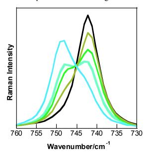
Figure II.32: Raman spectra of (1-x)(BMI-TFSI), xLiTFSI ionic liquids for x = 0 (black), 0.08, 0.18, 0.22 and 0.36 (blue) by order of decreasing intensity at 742 cm<sup>-1</sup> and of increasing intensity at 748 cm<sup>-1</sup>, respectively. For a convenient comparison, all the spectra were normalized with respect to their total intensity integrated between 775 and 717 cm<sup>-1</sup>.
