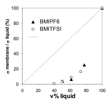
Figure II.25: Variation of  $\sigma_{membrane}/\sigma_{liquid}$  as compared to the volume % of liquid in the membrane for x LiTFSI = 0.03.
