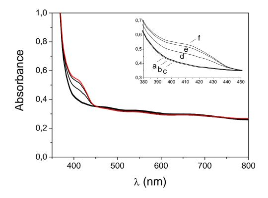
Figure III.30: Spectroelectrochemistry of the InHCF thin film of 5 mC/cm² on ITO/Orma, measure of the absorbance as a function of the applied potential, ref: Ag/AgCl, counter electrode: Pt foil; a)-1.0V, b) -0.5V, c) 0.0V, d) 0.5V, e)1.0V, f) 1.3V (as-deposited).
