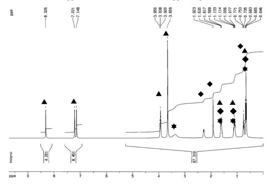
Figure II.48: ¹H NMR spectra of 0.3 LiTFSI / 0.97 BMITFSI with 20 wt% PMMA with reference D<sub>2</sub>O/MeOH at 50°C, ▲ BMI; **\*** PMMA; ◆ Butanone
