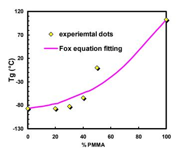
Figure II.6: Variation of the glass transition temperature (Tg) of membranes containing 0.03LiTFSI/0.97BMITFSI with respect to the PMMA weight percentage (from 0 to 50%), and comparison with Fox equation.
