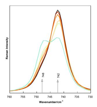
Figure II.38: Raman spectra of PMMA membranes plasticized by (1-x) (BMI-TFSI), xLiTFSI with x = 0.23. The quantity of PMMA is 0, 10, 20, 30, 40 and 50 wt% by order of increasing intensity at 742 cm<sup>-1</sup>, respectively. All the spectra have been normalized by integration between 775 and 717 cm<sup>-1</sup>. A fitting of the two components has been performed using mixed Gaussian/Lorenzian profiles with the proportion of Lorentzian up to 60%, as illustrated in Figure II.39 for 40 wt% PMMA.
