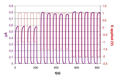
Figure IV.12: Spectroelectrochemistry of the following complete device: Glass/ FTO/ PEDOT Orgacon / electrolytic membrane : 70% 0.03 LiTFSI/ 0.97 BMITFSI, 30% PMMA / BP / FTO/Glass, measure of the  $\Delta A$  while applying colouring and bleaching potentials.
