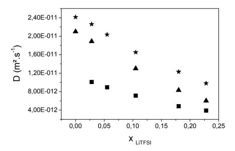
Figure II.51: Diffusion coefficients measured by PGSE-NMR, dependence on the LiTFSI molar ratio at 25°C for:  $\star^{1}$ H,  $\Delta^{19}$ F,  $\blacksquare^{7}$ Li.
