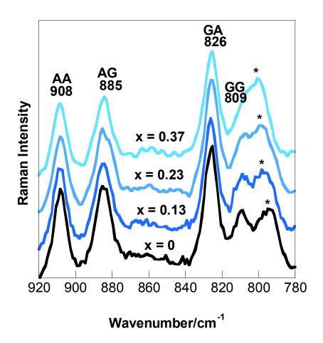
Figure II.31: Raman spectra of (1-x)BMITFSI,xLiTFSI ionic liquids at 298 K. The asterisk indicates a band of the anion, all the other bands being due to the indicated BMI<sup>+</sup> conformers.
