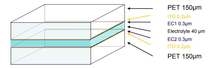
Figure II.1: Complete EC device and the approximate dimensions for each layer of the stack, the electrolyte has a central position.
