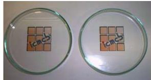
Figure II.7: Two Petri dishes: left hand side with no deposited membrane and right hand side with an electrolytic membrane (0.03 LiTFSI/0.97 BMITFSI) for a PMMA 30 wt %.
