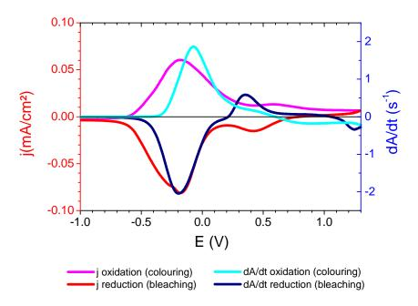
Figure III.27: Cyclic voltammetry at 8.3 mV/s, j = f(V) on the left axis and cyclic volta-absoptometry dA/dt = f(V) at 720 nm on the right axis for Prussian Blue on FTO/glass at 3 mC/cm<sup>2</sup>, reference electrode CSE, counter electrode FTO/glass.
