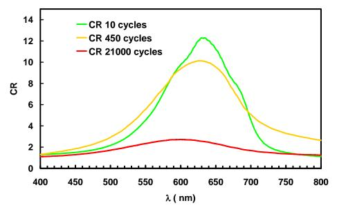
Figure IV.27: Contrast ratio of a complete device with 12\*15 cm<sup>2</sup> active area in the 400-800 region as a function of the applied potential. The absorbance measurement were performed at -1.3 V for the colouration and +1.0 V for the bleaching after 10, 450 and 21000 cycles.
