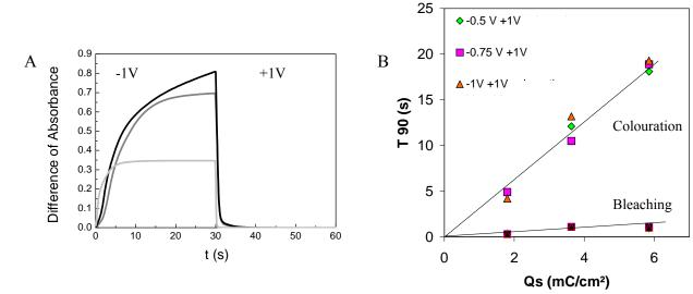
Figure III.13 : A. Difference of absorbance  $\Delta A$  between the coloured and bleached states with time for -1.0V applied for colouration during the first 30s., followed by 30s at +1V, light : 1.8 mC/cm², medium : 3.6 mC/cm², dark : 5.9 mC/cm². B. Response time to obtain 90 % of colouration or bleaching (T90) as a function of the capacity of the films for different applied potentials in colouration (-0.5 V; -0.75 V and -1.0V), the bleaching potential remains 1.0V, at  $\lambda$ =610 nm.
