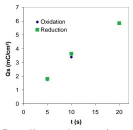
Figure III.10 : Evolution of the film capacities, measured at a constant low current density (15  $\mu$ A/cm²) between -1.0 V and +1.0 V vs. Ag/AgCl, as a function of the film-deposition time "t" for films EP1 (5 s), EP2 (10 s) and EP3 (20 s)
