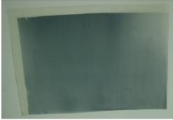
Figure IV.4: Photo of a PEDOT on ITO/PET prepared at ISC (11\*15cm² active surface)
