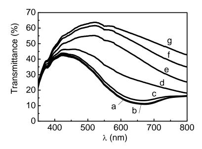
Figure IV.11: UV-Visible spectra during spectroelectrochemical study of a complete device (30 wt% PMMA/70wt% 0.03 LiTFSI- 0.97 BMITFSI), in the 400-800 region as a function of the applied potential. Transmittance measured at. a) -1.8 V, b) -1.5 V, c) -1.0 V, d) -0.5 V, e) 0.0V, f) 0.5 V, g) 1.0 V, air is taken as the reference.
