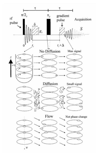
Figure II.49: A schematic representation of how the Stejskal and Tanner or PFG pulse sequence measures diffusion and flow. Reprinted from ref 44.
