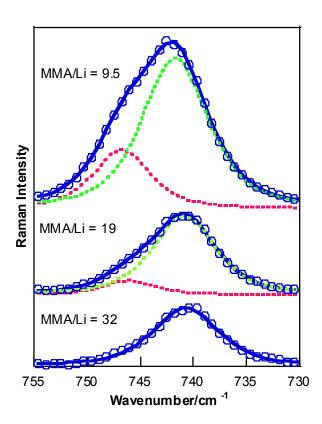
Figure II.36: Raman spectra focussed on the TFSI bands at 742 and 747 cm<sup>-1</sup> of LiTFSI/PMMA blends with composition MMA/Li = 32, 19 and 9.5, fitted as described in the text.
