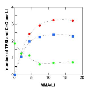
Figure II.41: Population of coordinated anions ( $\bullet$ ) per lithium and number of coordinated C=O groups per lithium ( $\bullet$ :  $R_{IR} = 1.0$ ,  $\blacksquare$ :  $R_{IR} = 1.5$ ) as a function of the number of polymer repeat units per lithium, MMA/Li, for a composition x = 0.23 in  $(1-x)(BMI-TFSI)_xLiTFSI$ .
