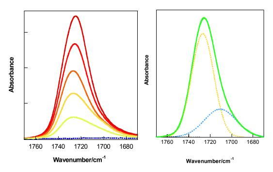
Figure II.40: a) FTIR-ATR spectra at room temperature of PMMA membranes plasticized by (1-x)(BMI-TFSI),xLiTFS<sub>I</sub> with x = 0.23, with increasing quantities of PMMA as follows: 0 (dotted blue line, pure ionic liquid), 10, 20, 30, 40 and 50 wt% from bottom to top.
