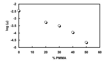
Figure II.24: Variation of  $\log (\sigma)$  at 30°C with the wt% of PMMA in the membrane for x = 0.03 in BMITFSI.
