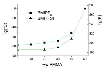
Figure II.5: Variation of the glass transition temperature (Tg) of membranes containing  $0.04 \text{LiTFSI}/0.96 \text{BMIPF}_6$  and 0.03 LiTFSI/0.97 BMITFSI with respect to the PMMA weight percentage (from 0 to 50%) in the membrane.
