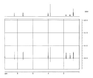
Figure II.50: 2D representation of chemical displacement in X-coordinate and diffusion coefficient ( $10^y$ ) in Y-coordinate for a LiTFSI/BMITFSI solution ( $x_{LiTFSI} = 0.03$ )
