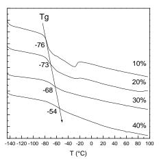
Figure C.1 : Evolution of the DSC curves with increasing PMMA wt% from 10 to 40 in xLiTFSI/(1-x)BMIPF<sub>6</sub> x = 0.04.
