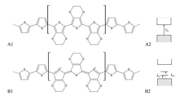
Figure III.2: Neutral PEDOT formula (A1) and its band gap structure (A2). Bipolaronic species obtained via two-electron oxidation (p-doping): formula (B1) and band gap structure (B2).
