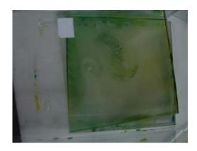
Figure E.3: Unsuccessful trial of electrochemical bleaching (counter-electrode: FTO, pseudo-reference electrode: Ag/AgCl), potential applied up to -2V.
