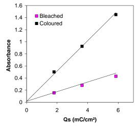
Figure III.11: Evolution of the films maximum absorbance with the film capacity for the films EP1 (5 s), EP2 (10 s) and EP3 (20 s).
