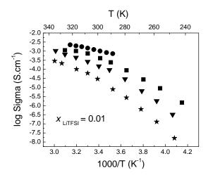
Figure C.10: Temperature dependence of the ionic conductivity σ for BMIPF<sub>6</sub> electrolytes with LiTFSI molar ratio of 0.01 and PMMA wt%: • 0%; ■ 20%; ▼ 30%; ★ 40%
