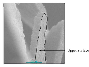
Figure III.25 : SEM images of the surface of InHCF films deposited by cyclic voltammetry for 150 cycles on FTO/glass, cracks on the InHCF films have been intentionally made to observe the surface and the side of the film, 6.5 mC/cm<sup>2</sup>.
