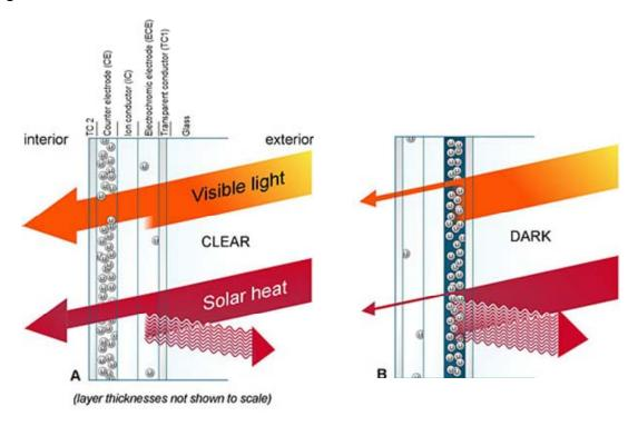
Diagram of a typical electrochromic coating<sup>1</sup>.
