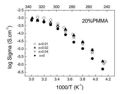
Figure C.6: Temperature dependence of the ionic conductivity  $\sigma$  for BMIPF<sub>6</sub> electrolytes with 20 wt% PMMA and LiTFSI molar ratio: • 0.00,  $\bigcirc$  0.01,  $\blacktriangle$  0.02,  $\leftrightarrows$  0.04.
