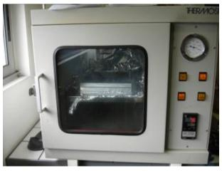
Figure IV.8: Hot-pressing of the whole stack under vacuum at 80°C for at least 2h.
