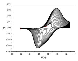
Figure III.21: Electrodeposition of InHCF on FTO/glass by cyclic voltammetry at 100 mV/s between 0.2V and 1.3 V/SCE, counter electrode FTO/glass, 50 cycles, 4\*5 cm<sup>2</sup>.
