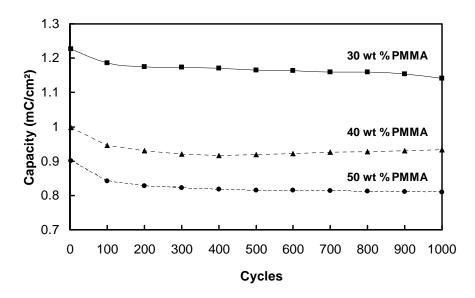
Figure IV.15: Variation of the capacity during cycling at -1V 5 s +1V 5 s. of devices with 30 to 50 % PMMA in 0.03 LiTFSI / 0.97 BMITFSI
