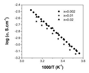
Figure C.3 : Temperature dependence of the conductivity  $\sigma$  in the range -30°C - +60°C for BMIPF<sub>6</sub> solutions with LiTFSI molar fractions: • 0.002;  $\star$  0.01; • 0.02.
