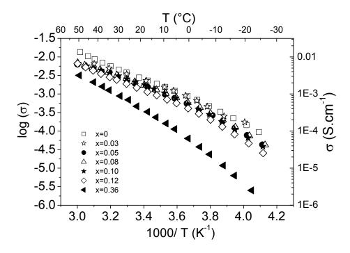
Figure II.14: Temperature dependence of the conductivity  $\sigma$  in the range -30°C - +60°C for BMITFSI solutions with LiTFSI molar fractions x:  $\Box$  0.0;  $\diamondsuit$  0.03;  $\bullet$  0.05;  $\triangle$  0.08;  $\star$  0.10;  $\diamondsuit$  0.12;  $\blacktriangleleft$  0.36.
