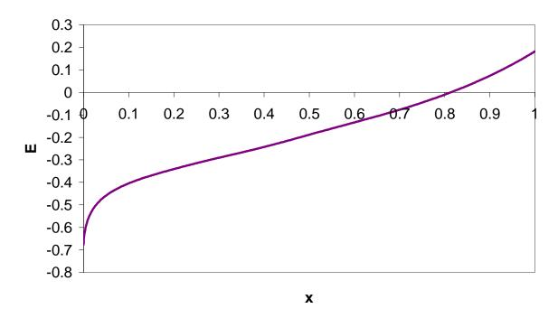
Figure F.1: Chronopotentiometric curves for the first oxidation at low current density (1  $\mu$ A/cm<sup>2</sup>) of PB 3 mC/cm<sup>2</sup> in a 0.03 LiTFSI/ 0.97 BMITFSI.
