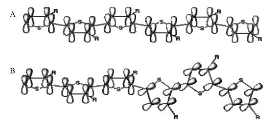
Figure III.3: Undoped (A) and p-doped (B) PEDOT molecular orbital schematization
