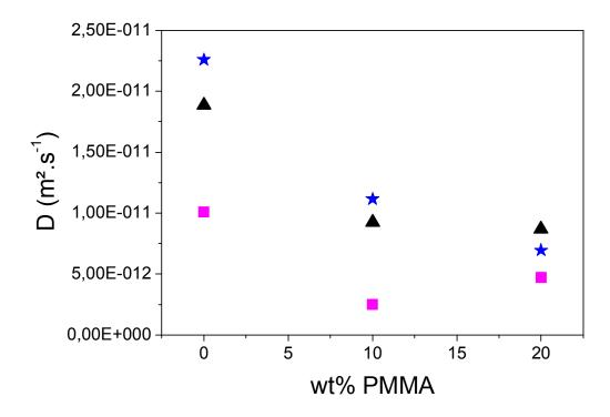
Figure II.53: Diffusion coefficients measured by PGSE-NMR as a function of wt% PMMA in (1-x)(BMITFSI), xLiTFSI (x=0.03) ionic liquids at 25 °C:  $\star$ : <sup>1</sup>H,  $\Delta$ : <sup>19</sup>F,  $\blacksquare$ : <sup>7</sup>Li
