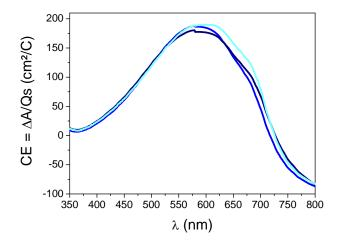
Figure III.12 : Variation of the colouration efficiency with  $\lambda$  as the film capacity increases from 1.8 mC/cm<sup>2</sup> (EP1, 5 s deposition) to 5.9 mC/cm<sup>2</sup> (EP3, 20 s deposition)
