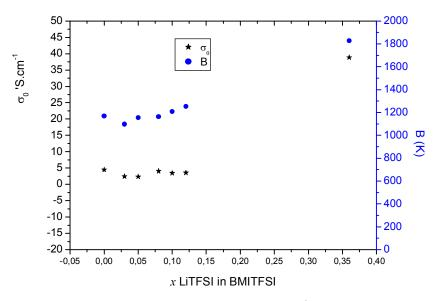
Figure II.17: Variation of  $\sigma_0$  and B with the amount of Li<sup>+</sup> salt in BMITFSI.
