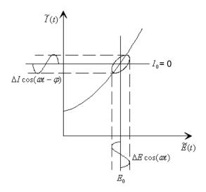
Figure II.10: Principle of EIS, a periodic signal is applied to the sample and the periodic variation of the studied parameter is measured.
