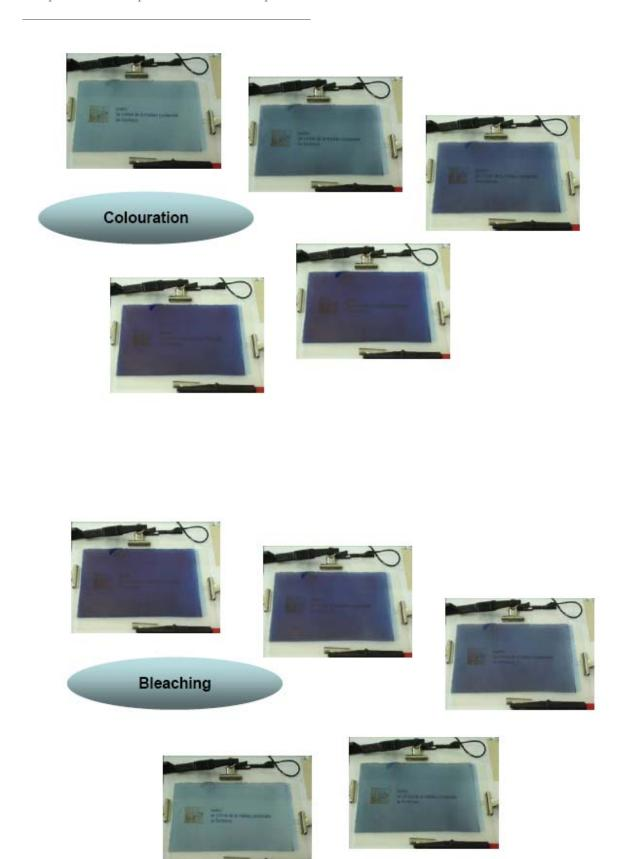
$\label{eq:Figure IV.20} Figure\ IV.20: Bleached\ to\ fully\ coloured\ state\ of\ the\ complete\ device\ (and\ reverse)\ ,\ showing\ the\ control\ of\ light\ shading\ with\ potential.$
