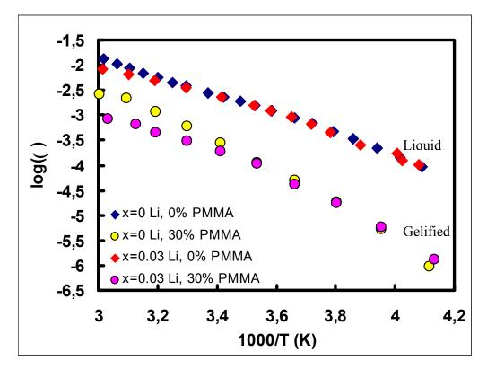
Figure II.18: Temperature dependence of the ionic conductivity  $\sigma$  in the range -30°C - +60°C for BMITFSI ( $\blacklozenge$ ), BMITFSI with 30 wt% PMMA ( $\blacklozenge$ ), BMITFSI with 0.03 LiTFSI ( $\blacklozenge$ ), and BMITFSI with 0.03 LiTFSI and 30 wt% PMMA ( $\blacklozenge$ ).
