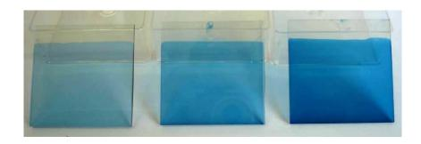
Figure III.20 : Prussian Blue films electrodeposited on FTO/glass ( $R_{\Omega/\square} = 13$ ) with capacities of 3, 6 and 12  ${}^{\text{mC/cm}^2}$
