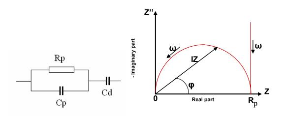
Figure II.11: RpCp electrical circuit with Cd capacity from blocking electrode (a) and associated Nyquist plot (b).
