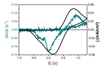
Figure III.31: Volta-absorptometry of a 5 mC/cm<sup>2</sup> InHCF deposited on ITO/Orma at 8.3 mV/s at 420 nm.
