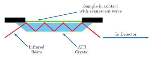
Figure A.4 : Total internal reflection at the interface between the ATR crystal and the sample. Depth of penetration of the evanescent wave is approximately 1  $\mu$ m
