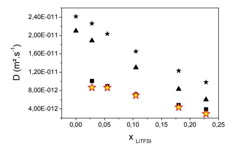
Figure II.52: Diffusion coefficients measured by PGSE-NMR as a function of x in  $(1-x)(BMITFSI)_xLiTFSI$  ionic liquids at 25°C: black stars:  $^1H$ , triangles:  $^{19}F$ , squares:  $^7Li$ , red stars:  $^{19}F$  diffusion coefficient of the coordinated anions in Li(TFSI)<sub>2</sub>-, calculated as explained in the text.
