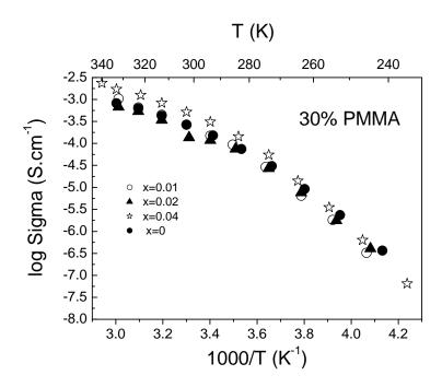
Figure C.7: Temperature dependence of the ionic conductivity  $\sigma$  for BMIPF<sub>6</sub> electrolytes with 30wt% PMMA and LiTFSI molar ratio:  $\bullet$  0.00,  $\bigcirc$  0.01,  $\blacktriangle$  0.02,  $\stackrel{\checkmark}{\bowtie}$  0.04
