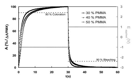
Figure IV.14 : Kinetics of colouration and bleaching at 610 nm when switching the potentials at -1.0V for colouring and +1.0V for bleaching.
