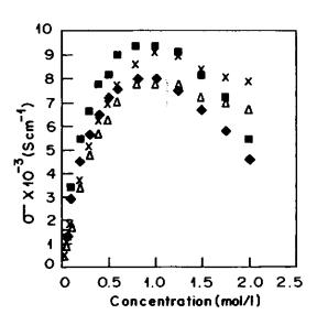
Figure B.1 : Evolution of the conductivity at 25°C as a function of LiClO<sub>4</sub> and LiN(CF<sub>3</sub>SO<sub>2</sub>)<sub>2</sub> concentration in PC( $\blacklozenge$ , $\Delta$ ) and PC+EC( $\blacksquare$ ,  $\times$ ), respectively. Reprinted from reference 5
