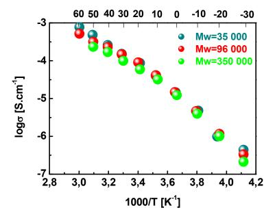
Figure II.19: Temperature dependence of the ionic conductivity  $\sigma$  in the range -30°C - 60°C for different molecular weights of PMMA (30% PMMA membrane).
