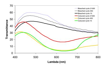
Figure IV.25: UV-Visible spectra during spectroelectrochemical study of a complete device with 12\*15 cm<sup>2</sup> active area in the 400-800 region as a function of the applied potential. Transmittance measured at -1.3 V for the colouration and +1.0 V for the bleaching after 10, 450 and 21000 cycles.
