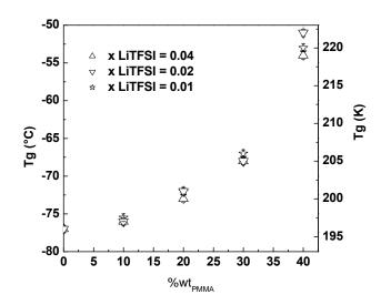
Figure C.2: Evolution of the glass transition temperature of the membranes containing x = 0.01 to 0.04 LiTFSI in BMIPF<sub>6</sub> with respect to the PMMA weight percentage (from 0 to 40%).
