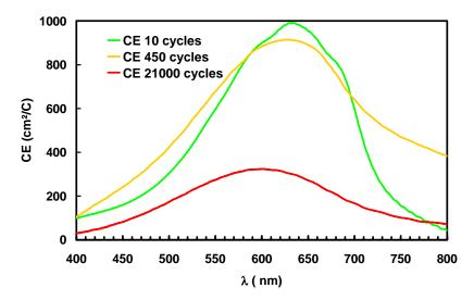
Figure IV.26 : Colouration efficiencies of a complete device with 12\*15 cm² active area in the 400-800 region as a function of the applied potential. The absorbance measurement were performed at -1.3 V for the colouration and +1.0 V for the bleaching after 10, 450 and 21000 cycles.
