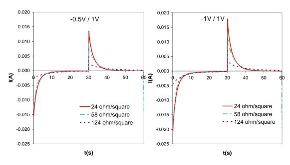
Figure IV.17: Variation of the current consumed by the device with time for EC devices prepared with conducting substrate of sheet resistance 24, 58 and 124  $\Omega/\Box$ : colouration at -0.5V (left) and at -1.0V (right) for 30 s. followed by bleaching at 1.0V the next 30 s..
