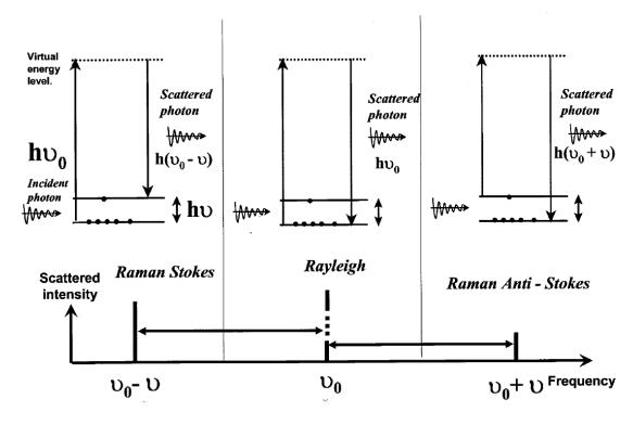
Figure A.3: Rayleigh, Stokes and Anti-Stokes scattering
