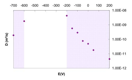
Figure F.3: Diffusion coefficient measured by EIS on a Prussian Blue sample at 3 mC/cm<sup>2</sup> on FTO/glass in 0.03 LiTFSI / 0.97 BMITFSI electrolyte. The purple zones correspond to the range of potentials for which the EIS spectra show diffusion Warburg slope.
