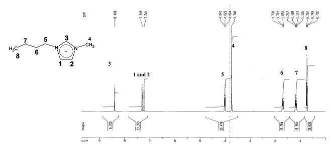
Figure II.44: <sup>1</sup>H NMR spectrum of 0.03LiTFSI/0.97BMITFSI in D<sub>2</sub>O/MeOH, and proton assignation.
