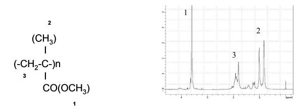
Figure II.47: <sup>1</sup>H NMR spectrum of PMMA dissolved in CDCl<sub>3</sub>. The peak assignation shows the atacticity of the PMMA.
