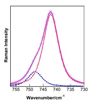
Figure II.39: Raman spectra of PMMA membranes (40 wt %) plasticized by  $(1-x)(BMI-TFSI)_xLiTFSI$  with x = 0.23. The two components have mixed Gaussian/Lorentzian profiles with a proportion of Lorentzian up to 60%.
