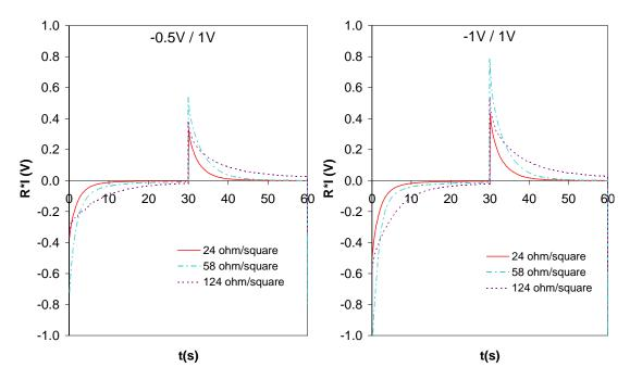
Figure IV.18: Variation of the product of the resistance of the device by the current passing through it with time for EC devices prepared with conducting substrate of sheet resistance 24, 58 and 124  $\Omega/\Box$ : colouration at -0.5V (left) and at -1.0V (right) for 30 s. followed by bleaching at 1.0V the next 30 s..
