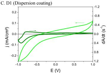
Figure III.14 : Cyclic voltammograms at 500 mV/min, and volta-absorptometry at  $\lambda$  max in 0.03/0.97 molar ratio LiTFSI/BMITFSI, in a three-electrode cell configuration for electropolymerised PEDOT EP2 (A) in-situ polymerized PEDOT ISP1 (B) , and PEDOT Orgacon D1 (C)
