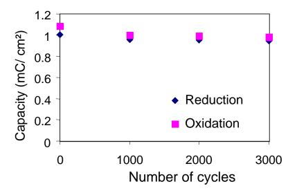
Figure IV.3 : Variation of the capacity of the device with the number of cycles measured by chornoamperometry while applying -0.5V / +1.0V.
