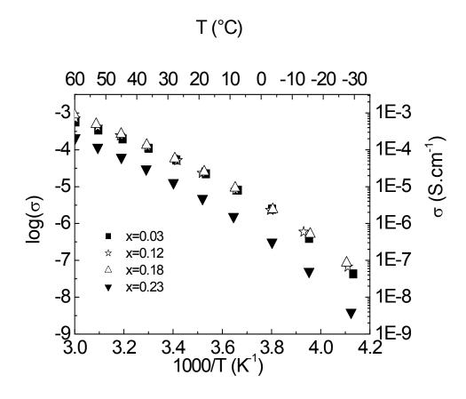
Figure II.20: Temperature dependence of the ionic conductivity  $\sigma$  in the range -30°C - +60°C for membranes consisting of PMMA (40 wt%) and BMITFSI solutions with LiTFSI molar fractions:  $x_{\text{LiTFSI}} = 0.03$ ; 0.12; 0.18 and 0.23.
