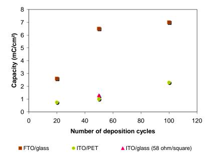
Figure III.22: Variation of the film capacity (measured by the area of the last oxidative scan during the deposition process) for FTO/glass, ITO/PET and ITO/glass substrates with the number of deposition cycles at 100 mV/s. The counter-electrode is an FTO/glass plate, the reference is a saturated calomel electrode (SCE).
