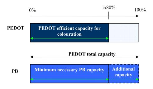
Figure IV.2 : PEDOT and Prussian Blue efficient capacity for colouration: for PB the whole capacity leads to colouration whereas for PEDOT it is only a part of it As-deposited PEDOT is slightly coloured (partly reduced). PB capacity must be chosen in between 77% and 100% of PEDOT capacity.
