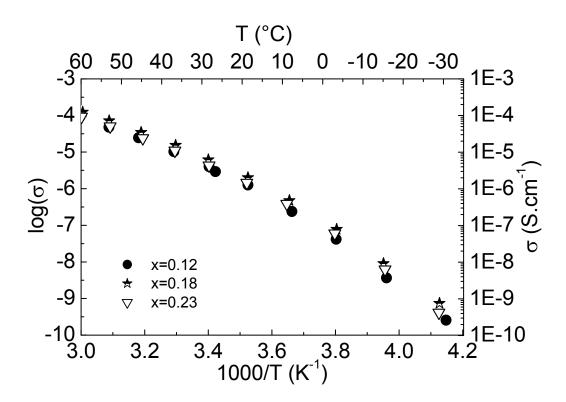
Figure II.21: Temperature dependence of the ionic conductivity  $\sigma$  in the range -30 °C - +60 °C for membranes with 50 wt % PMMA and BMITFSI solutions with LiTFSI molar fractions: 0.12; 0.18 and 0.23.
