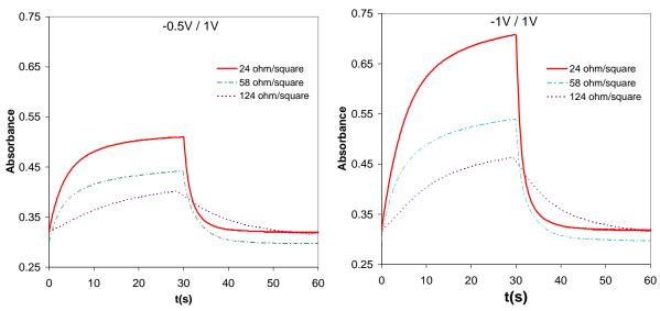
Figure IV.16 : Variation of the absorbance with time for EC devices prepared with conducting substrate of sheet resistance 24, 58 and 124  $\Omega/\Box$  : colouration at -0.5V (left) and at -1.0V (right) for 30 s. followed by bleaching at 1.0V the next 30 s..
