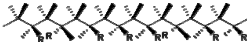
Figure D.4: Atactic polymer, random succession of mm , rr , rm triads
