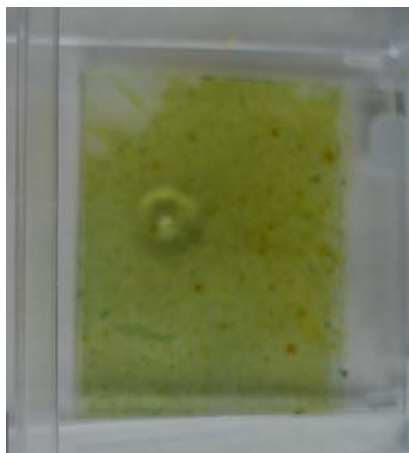
Figure E.2: Example of deposition using spin coating, 1000 pm, 30s.
