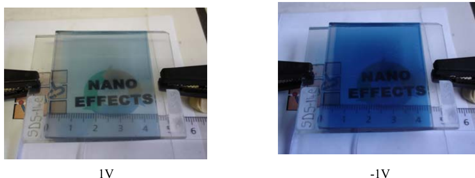
Figure IV.10 : Bleached (1V) and coloured state (-1V) of a -complete device with electrolytic membrane based on 70% LiTFSI 0.03 / BMITFSI 0.97 and 30 wt% PMMA, on FTO/glass with PEDOT PSS and PB electrochromic films.
