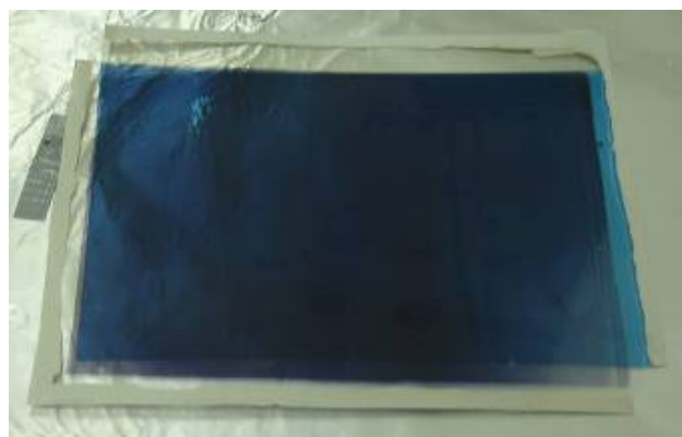
Figure IV.7: Application (manual lamination) of coloured PEDOT on the electrolyte/Prussian Blue stacks.
