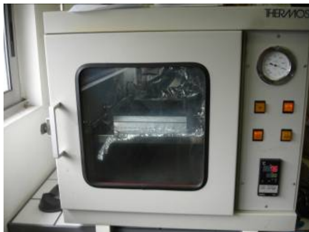
Figure IV.8 : Hot-pressing of the whole stack under vacuum at 80°C for at least 2h.
