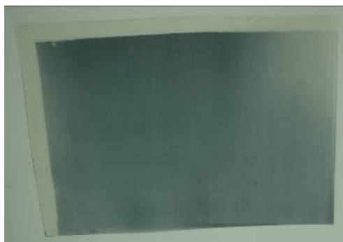
Figure IV.4 : Photo of a PEDOT on ITO/PET prepared at ISC (11*15cm 2 active surface)
