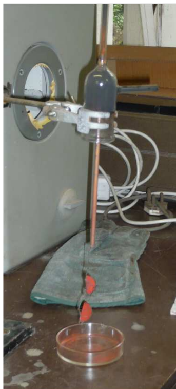
Figure 5.16: A hematite pellet before heating. The red fine rod is the thermocouple used to measure the temperature inside the furnace
