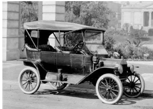
Figure 2: The first industrial use of steels with vanadium was to make the chassis of the Ford T.
