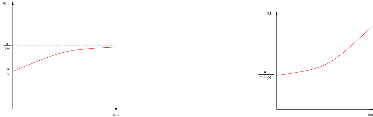
Figure 8.8: Behavior of the expectation E_J of the latency faced by a user job for a Pareto distribution of the grid latency. Left: no outliers ( \rho = 0 ); Right: \rho \neq 0 .
