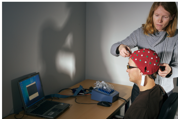
Figure 1.7: An EEG equipment : the electrode helmet is placed on the head of the subject, then the signal is processed through an amplifier and digitalized on a computer (Odyssee project team, INRIA Sophia Antipolis).
