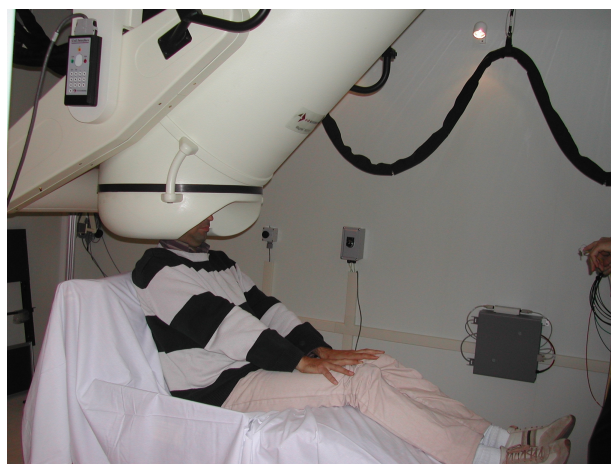
Figure 1.8: A MEG equipment : the helmet equipped with SQUID sensors is immersed in helium (Magnetoencephalography center, La Timone, Marseille).
