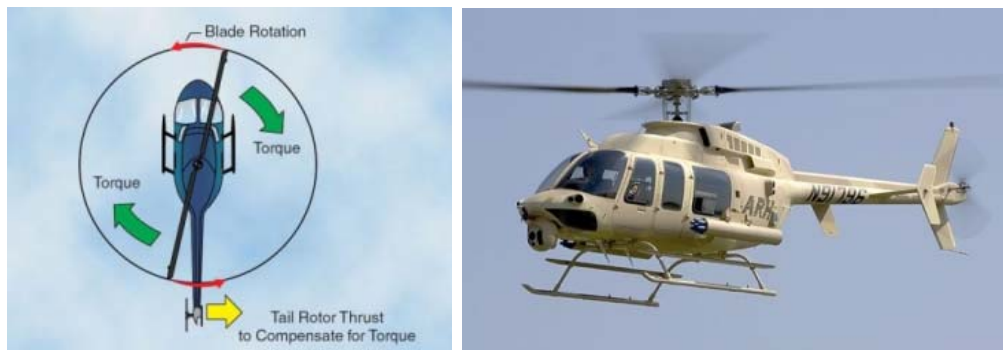
Figure 1.3: Helicopter with conventional tail rotor (source wikipedia ).
