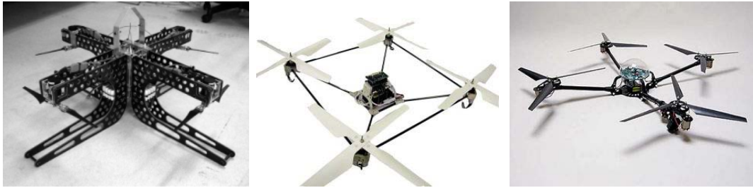
Figure 1.10: Reduced scale quadrotor helicopters developed by Australian National University, by the Centre d’Energie Atomique of France, and by Draganfly Innovations Inc.
