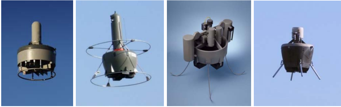
Figure 1.12: Ducted fan tailsitters: iSTAR, HoverEye, Honeywell, Goldeneye.
