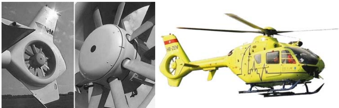
Figure 1.4: Fenestron and FANTAIL helicopter.
