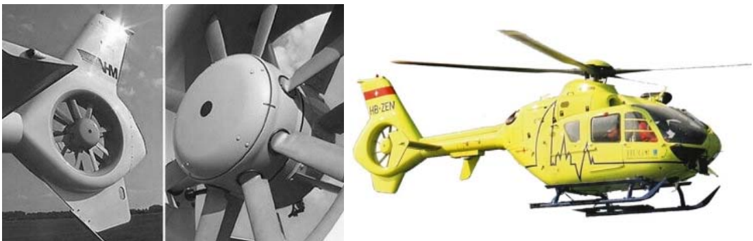
Figure 1.4: Fenestron and FANTAIL helicopter.
