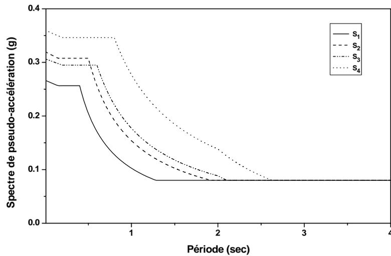
Figure A3.3: Spectres de calcul de EC8.
