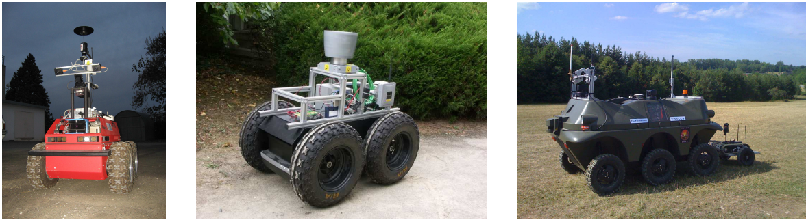
Figure 1: Three robots adapted to evolved in open and semi-structured terrains. From left to right: Dala and Mana from LAAS, respectively equipped with a stereovision bench and a panoramic Velodyne Lidar, and rTrooper from Thales TOSA, equipped with two stereovision benches.
