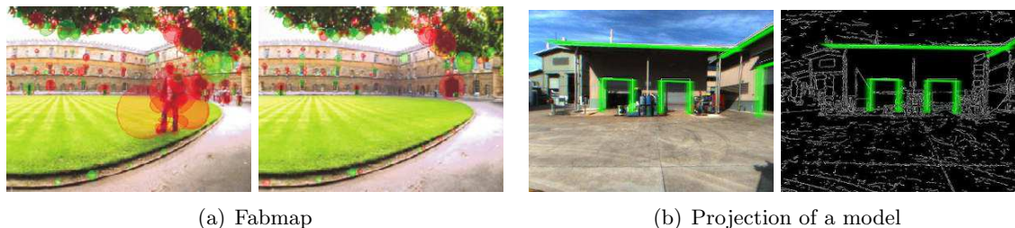
Figure 3.1: The two images of figure 3.1(a) are excerpts from [Cummins and Newman, 2008] and show a loop closure with scene changes, while figure 3.1(b) are excerpts from [Nuske et al., 2009] and show the projection of a model, green lines, on an image.
