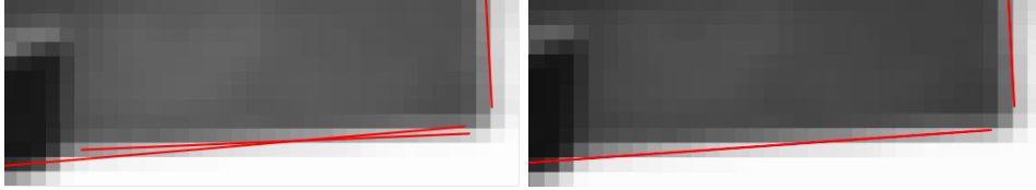
Figure 6.3: Line merging process. Left, two overlapping segments. Right, the line resulting from the merging process.
