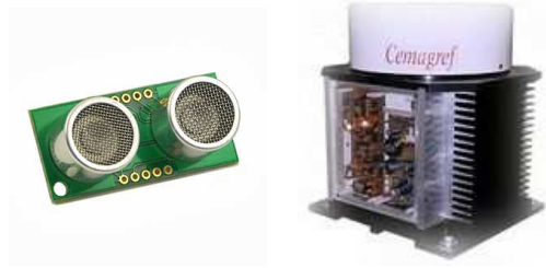
Figure 2.1: On the left, a cheap sonar, on the right the Cemagref's K2Pi Radar
