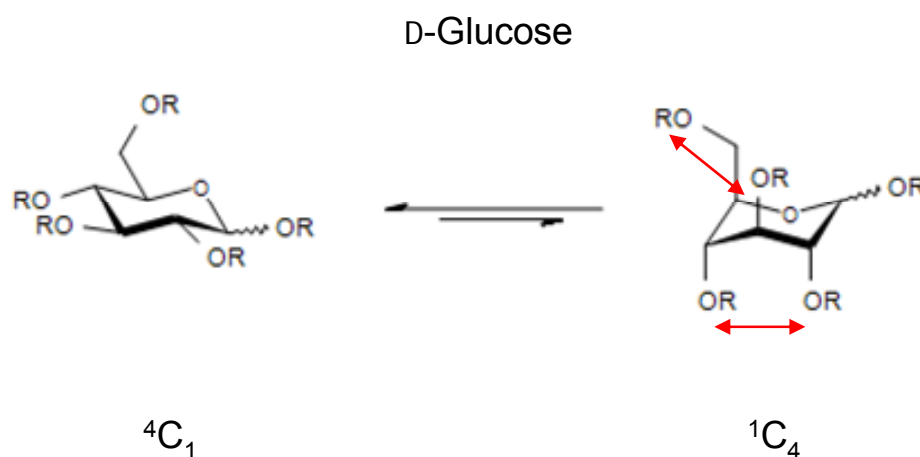
Figure 3 : Ring conformations of D-Glucose. {}^4C_1 is preferred over {}^1C_4 due to minimisation of 1-3 diaxial steric hindrance. This preference is increased upon increasing Van der Waals volumes of substituent R.
