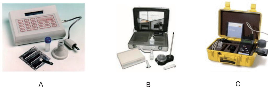
Figure 1.21: Three commercial portable apparatus for lead ion detection
