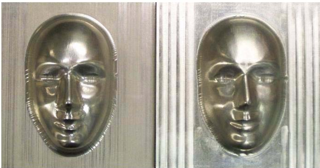
Figure 2.25 : Reverse Engineering (gauche), Copiage direct (droite)
