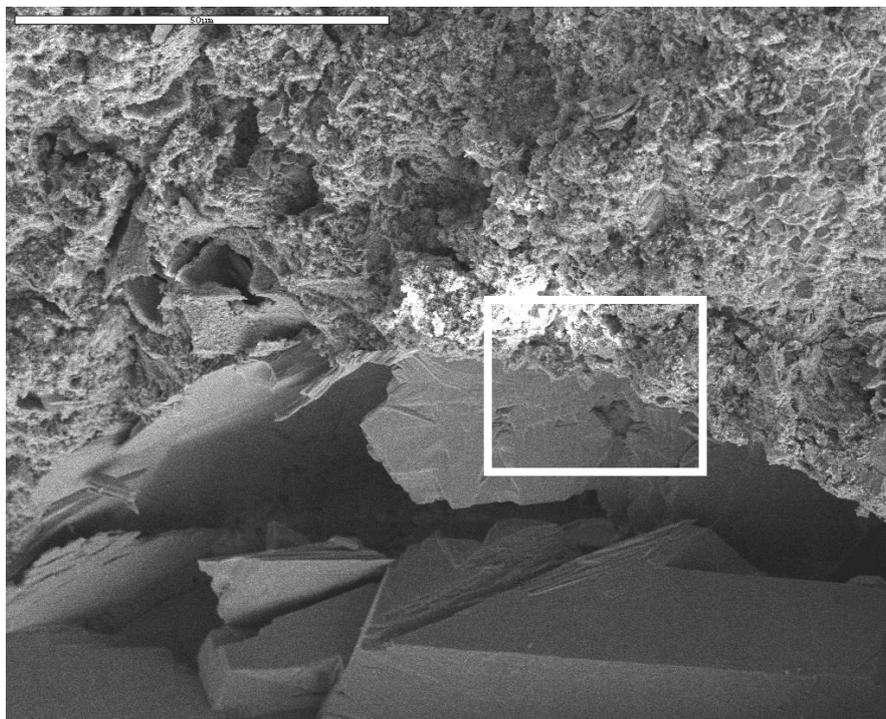
*Figure IV-34 : Fracture (x1000/5kv) - CEMII/59 Sain*
