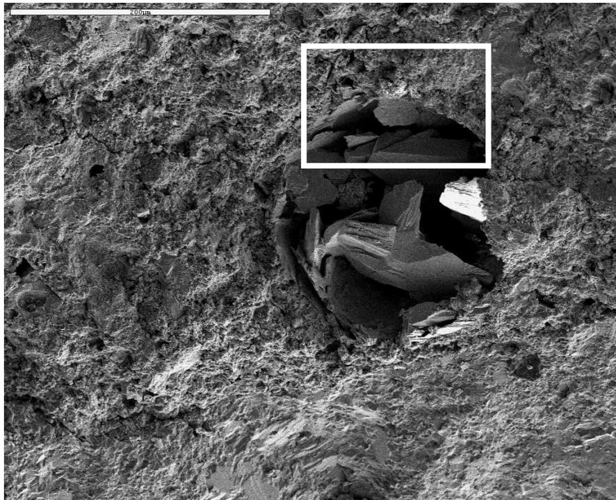
*Figure IV-33 : Fracture (x250/5kv) - CEMII/59 Sain*
