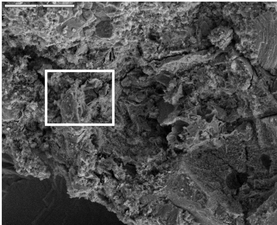
*Figure IV-35 : Fracture (x3000/5kv) - CEMII/59 Sain*
