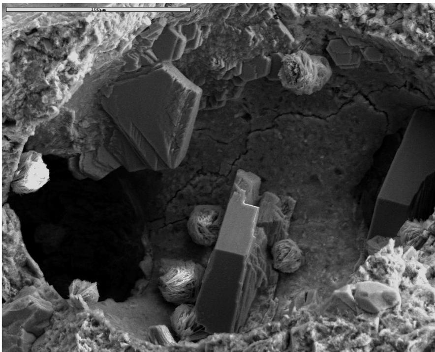
*Figure IV-56 : Fracture (x500/5kv) – CEM I/59 en I C*
