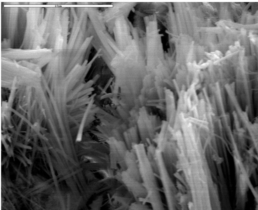
*Figure IV-51 : Fracture (x5000/5kv) – CEM II/49 en I C*
