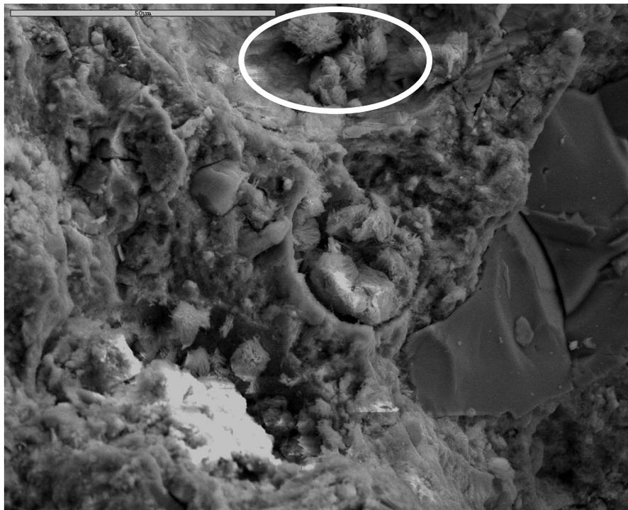
*Figure IV-60 : Fracture (x1000/5kv) – CEM I/49 en I C*
