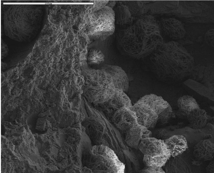
*Figure IV-54 : Fracture (x500/5kv) – CEM II/59 en I C*
