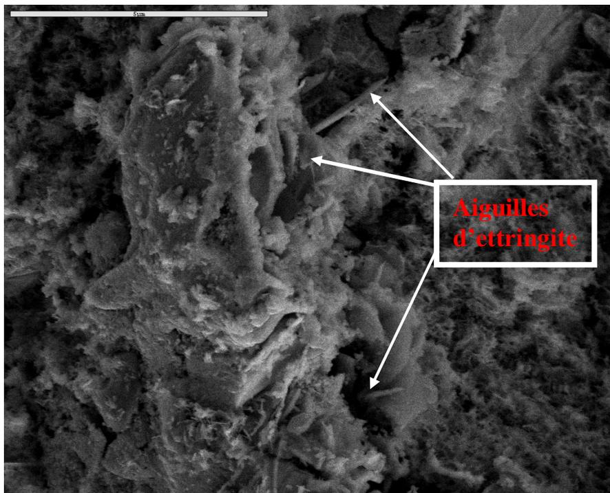
*Figure IV-36 : Fracture (x10000/5kv) - CEMII/59 Sain*
