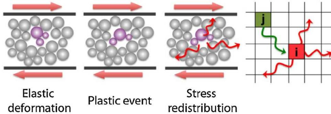
**FIG. 1.12** : Sketch of plastic deformation in amorphous media. Deformation occurs via elastic deformation, localized plastic events, and nonlocal redistribution of the elastic stress, potentially triggering other plastic events [65].
