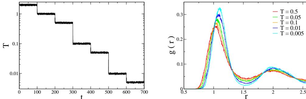
**FIG. 2.3** : **Left** : Temperature evolution during the quench protocol used to produce the Lennard-Jones glass samples. Time and temperature are expressed in LJ units. **Right** : Evolution during quench of the radial distribution function.
