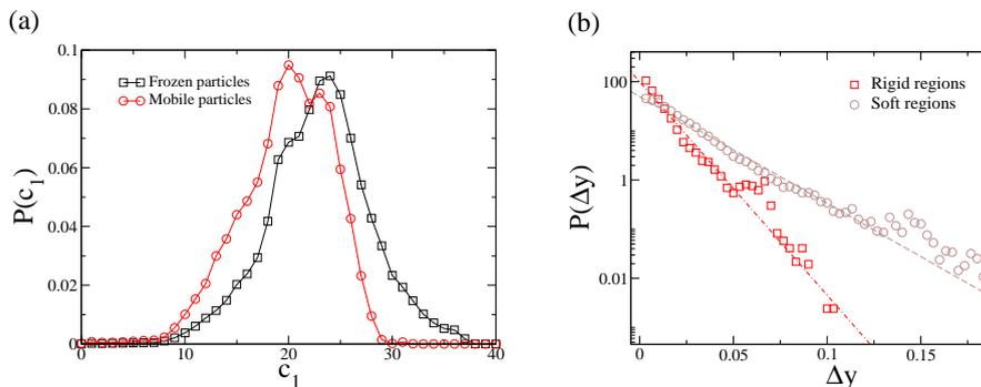
**FIG. 4.15** : (a) Distribution of the local shear modulus for mobile and immobile particles. (b) Distribution of the nonaffine field during a total strain of 1% for rigid and soft regions.
