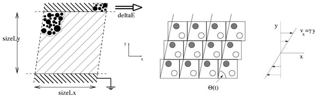
**FIG. 2.4** : **Left** : Schematic representation [117] of the quasistatic shearing protocol in two dimensions and under RWBCs. The bottom and top walls contain here frozen LJ particles, while the x direction remains periodic. **Right** : Schematic representation of the LEBCs.
