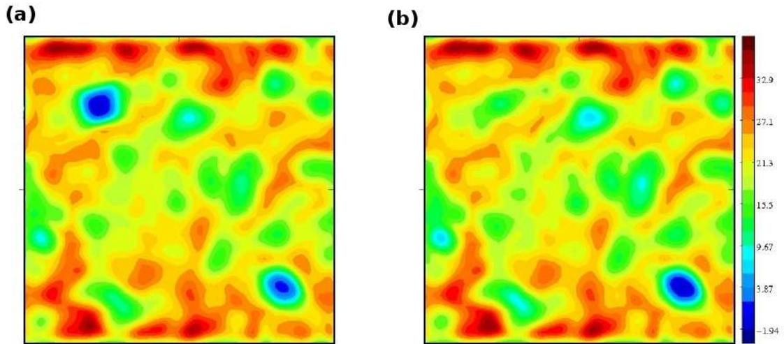
**FIG. 3.9** : Map of the local shear modulus for a coarse-grained length  $W = 5$  in the linear portion of the stress-strain mechanical response of the glass. (a)  $\varepsilon_{xy} = 0.27108\%$  just before a plastic event and (b)  $\varepsilon_{xy} = 0.2761\%$  just after the plastic event.
