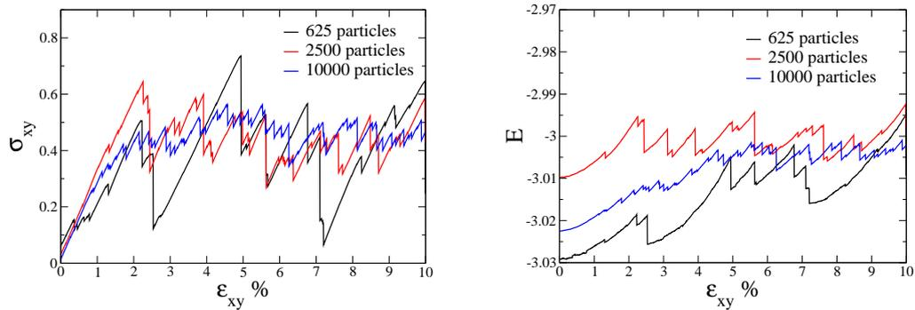
**FIG. 5.1** : **Left** : Stress-strain response of three two-dimensional polydisperse Lennard-Jones glass under Lees-Edwards boundary conditions. Each curve corresponds to a different square cell of size 25, 50 and 100 particle diameters. **Right** : Energy-strain mechanical response of the same samples. Here the total energy is divided by the total number of particles to produce the average energy per particle.
