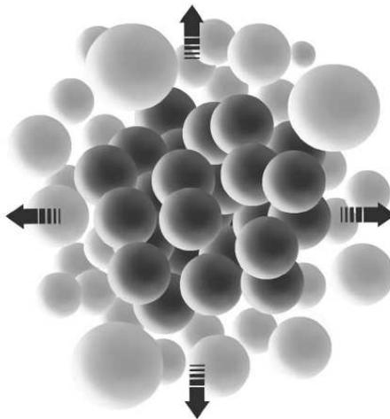
**FIG. 4.1** : A molecular rearrangement with the dark spheres showing molecules before the flow event. A flow event takes place if the region volume briefly expands sufficiently due to a thermal fluctuation. According to statistical mechanics the probability of this happening is the reversible work done on the surrounding fixed structure to bring about the same expansion [189].
