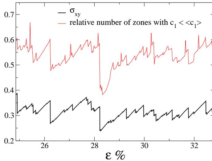
**FIG. 4.11** : Evolution of the total shear stress (thick line) and the relative number of soft zones (relative number of points  $\mathbf{r}$  where  $c_1(\mathbf{r}) < \bar{c}_1$ ) as a function of the applied shear strain, in the plastic flow regime.
