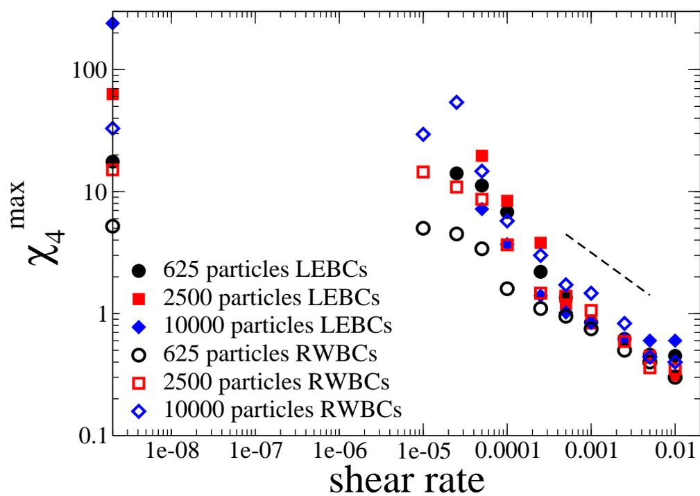
**FIG. 6.12** : maximum values  $\chi_4^{\max}$  of the four-point correlation function as a function of shear rate  $\dot{\gamma}$  for various system sizes and boundary conditions. The dashed line shows the power law  $\propto \dot{\gamma}^{-\mu}$ , with  $\mu = 0.6$ .
