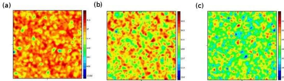
**FIG. 3.5** : The three eigenvalues of the elasticity tensor for a coarse-graining length  $W = 10$  on a square sample of size  $500 \times 500$  containing 226225 particles, (a)  $C_1$ , (b)  $C_2$ , (c)  $C_3$ .
