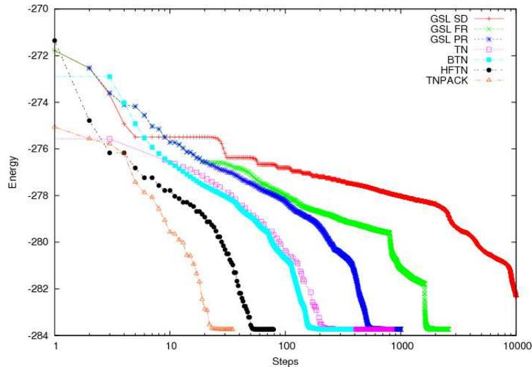
**FIG. 2.2**: Evolution of the energy of a Lennard-Jones glass sample containing 100 particles during energy minimization for various algorithms. From slowest to fastest, steepest descent algorithm (GSL SD) [84], Fletcher-Reeves conjugate gradient algorithm (GSL FR) [84], Polak-Ribiere conjugate gradient algorithm (GSL PR) [84], block truncated newton (BTN) [85], truncated newton (TN) [86], hessian free truncated method (HFTN) [87], truncated newton package (TNPACK) [88].
