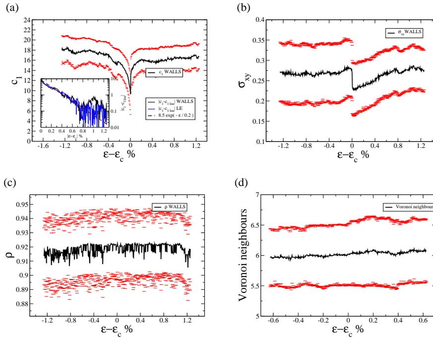
**FIG. 4.18** : Evolution of different fields around a plastic event and averaged over all plastic events. (a) local shear modulus, (b) local shear stress, (c) local density and (d) number of Voronoi neighbors.
