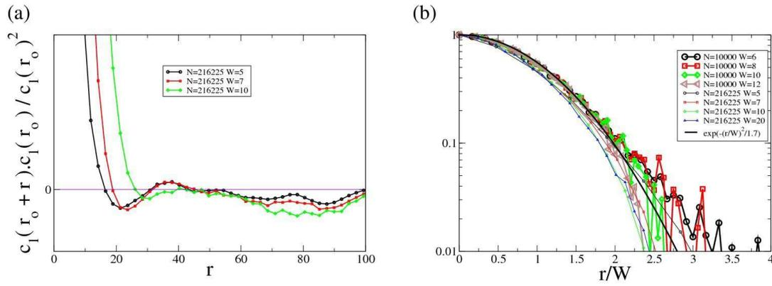
**FIG. 3.10** : (a) Spatial correlation function of the local shear modulus  $c_1$ :  $\langle (c_1(0) - \bar{c}_1)(c_1(r) - \bar{c}_1) \rangle$ .
