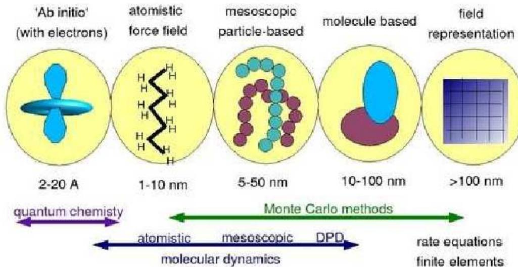
**FIG. 2.1** : Schematic representation of various modeling numerical methods as a function of the length scales of interest. We will place ourselves in the mesoscopic range adapted to the use of the Molecular Dynamics technique (H. Meyer Strasbourg).
