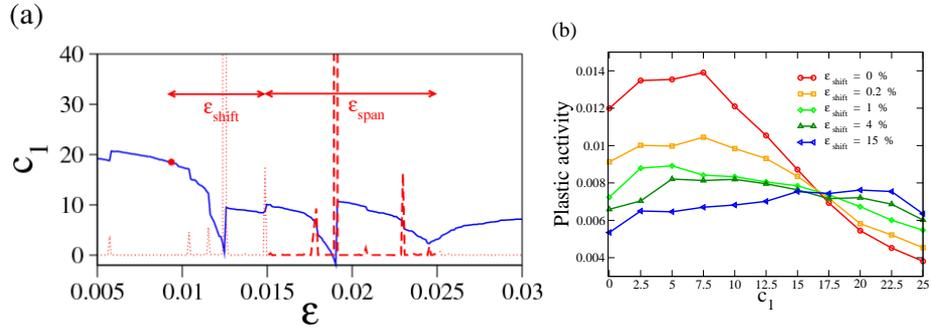
**FIG. 4.17** : (a): Evolution of  $c_1$  of a particle in a plastic zone. The dotted line represents the parameter  $D_{BF}$  that marks the local deviation from affinity.  $\varepsilon_{shift}$  and  $\varepsilon_{span}$  are defined for the point marked in red. (b): cumulative plastic activity for  $\varepsilon_{span} \sim 0.5\%$  and for different values of  $\varepsilon_{shift}$ .
