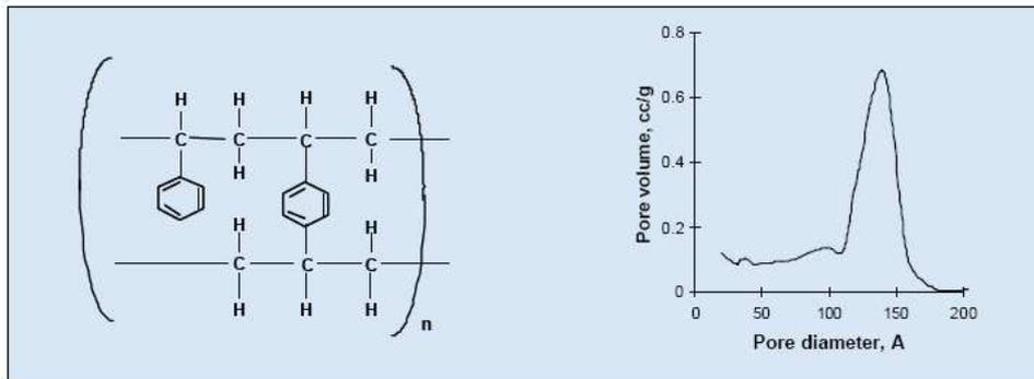
Figure 2 : Pore distribution of AMBERLITE XAD4 polymeric adsorbent
