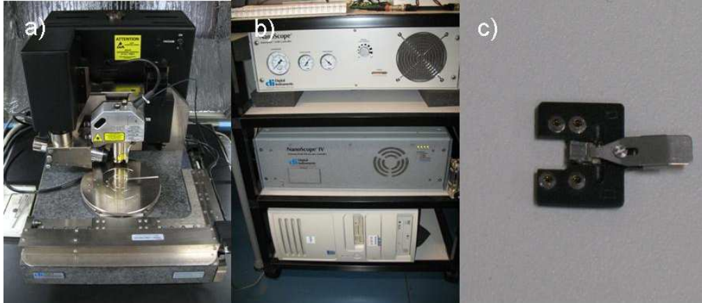
Figure 1.21 Dimension microscope and equipment: a) main microscope with anti-vibrating table, b) controllers, c) support for cantilever.
