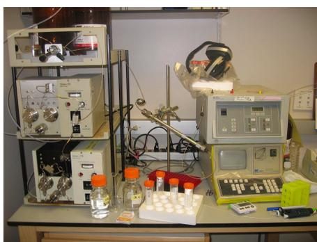
Figure 2.1: Gradient liquid chromatography apparatus.
