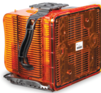
FIG. 1.3 – A 25-wafer lot for 300 mm processing
