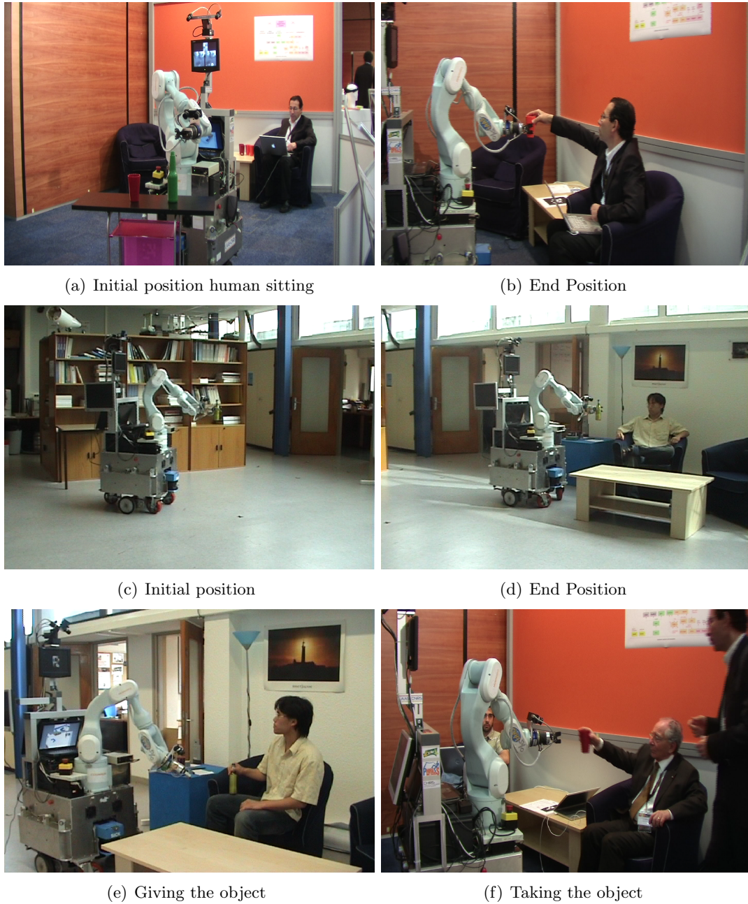
Figure 4.14: PSP to hand an object to a human sitting in front of a table a) and c) Initial positions, b) and d) Final configurations looking at the human. The robot is perceiving human by cameras on top. The robot finds its final configuration to complete the tasks of giving e) or taking f) the object.
