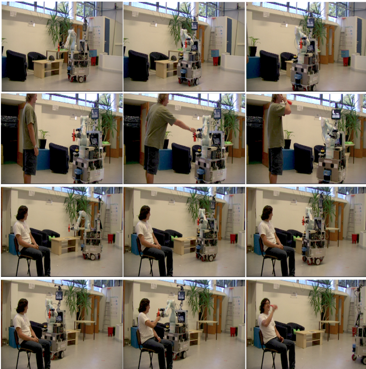
Figure 4.10: A whole “Fetch and carry” scenario, sequence where a robot has GoTo-Give task to a person that is standing and to a person that is sitting. We can see the difference on the approaching behavior of the robot. On the second case the robot takes into account that the human is in a sitting position but also the closest position to the robot current placement.
