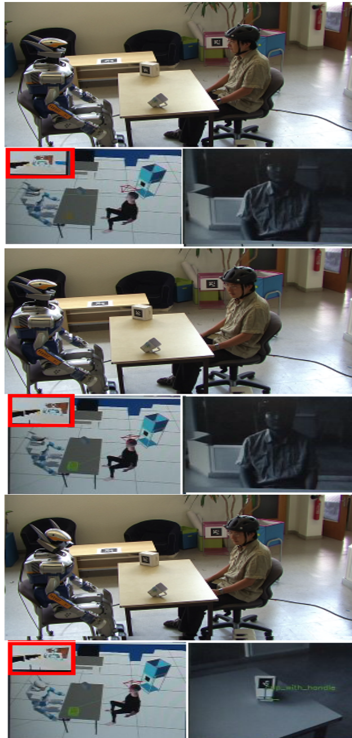
Figure 5.12: Scenario 1: the robot looks to the object that the human is looking. In the images: The scenario (up), the GEO-Move3D interface showing the process and the attentional object marked with a green grid box around the object (down-left) and robot's camera (down-right)
