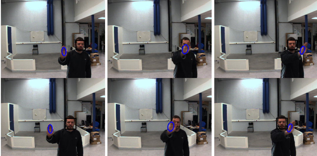
Figure 4.7: Hand being tracked by the Gest module : the ellipses are the projection of the 3D state vector
