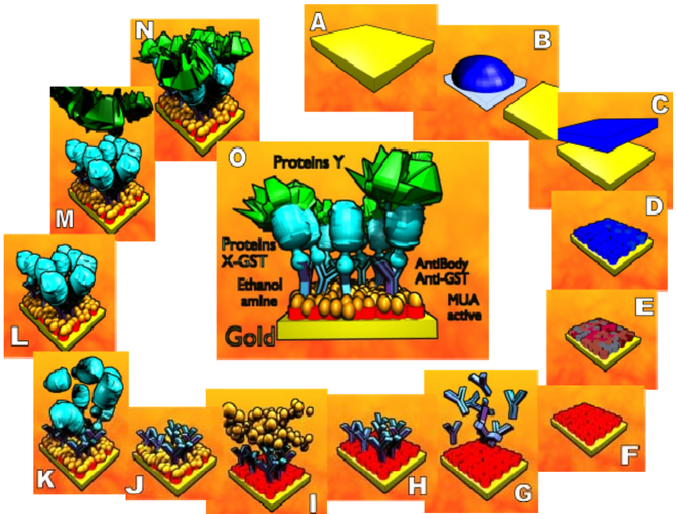
Figure 12: The different steps of the biochip sensor protocol. A: A thin layer of gold serves as a basis for the fixation of all the molecular architecture. B: A PDMS stamp is inked for 5 minutes with a 11-mercaptoundecanoic acid solution in ethanol. C: The stamp is dried and brought into contact with the gold sensor for 5 minutes. D: The surface is rinsed several times by ethanol and milliQ water. E: A mixture of NHS/EDC solution is incubated on the surface. F: The COOH group of the thiol molecules is changed into an active ester. G: An Anti-Gst antibody is covalently bounded on the surface. H: Saturation of the sensor surface with antibody is achieved in 45 minutes. I: An ethanolamine solution then passivates the surface. J: Since all the surface is saturated, we wash several times the sensor in order to remove loosely bounded molecules from the sensor. K: the first Gst-tagged proteins now interact with the antibody. L: We wash for removing all non bounded molecules. M: The second protein is injected. N: ...and can interact with the probe protein fixed on the surface.
