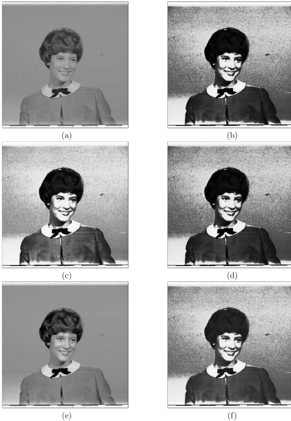
Figure 3.1: An example illustrates the CHE and Bi-HE methods for image brightness preserving and contrast enhancement may fail when producing natural looking images: (a) original image; enhanced images using (a) as input by CHE, BBHE, DSIHE, RMSHE ( r = 2 ), and MMBHEBE methods are shown in (b), (c), (d), (e), and (f), respectively.
