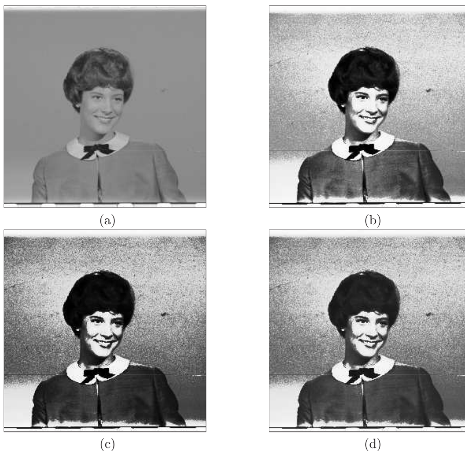
Figure 1.3: Bi-HE methods and still not natural looking images: (a) original image; enhanced images using (a) as input by [51]-(BBHE), [126]-(DSIHE), and [17]-(MMBHEBE) methods are shown in (b), (c), and (d), respectively.
